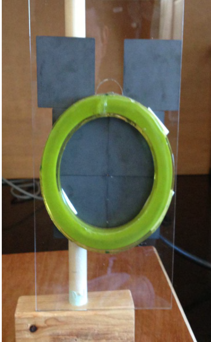
Figure 24. Photograph of the ferrite board behind the receiving coil.
