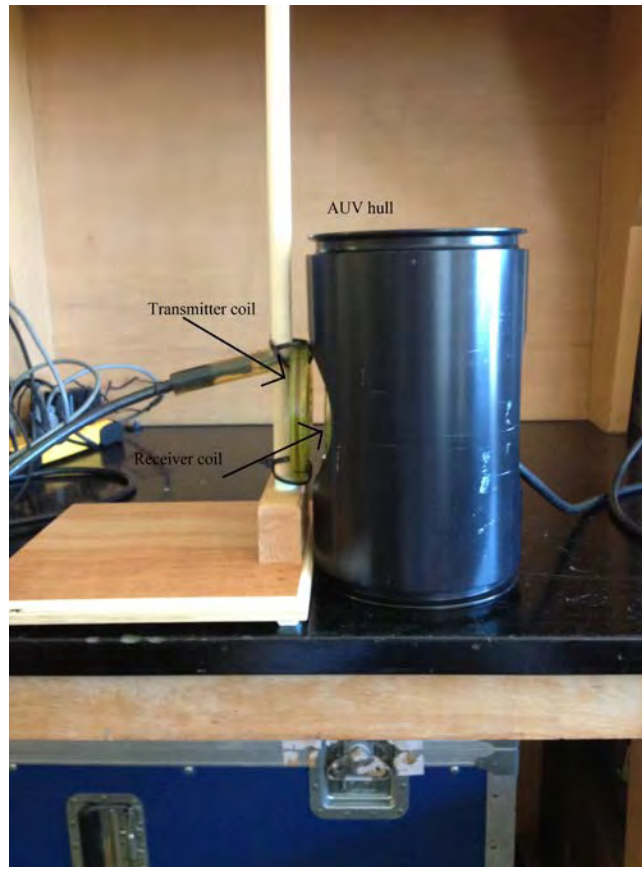
Figure 5 Setup of the transmitting coil and receiving coil with ferrite tiles placed inside an AUV hull.
