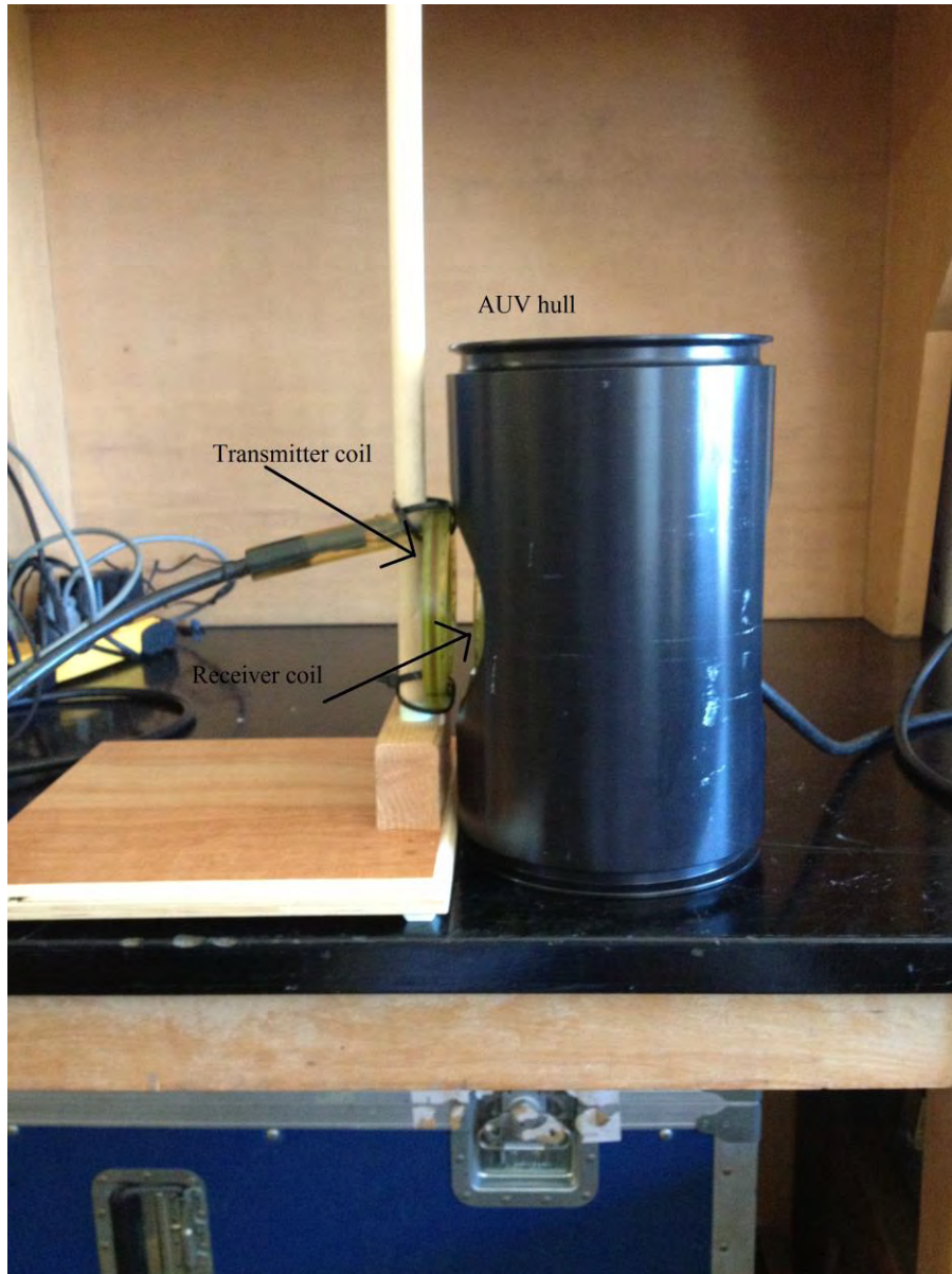
Figure 28. Setup of the transmitting coil and receiving coil with backing plate inside an AUV hull.
