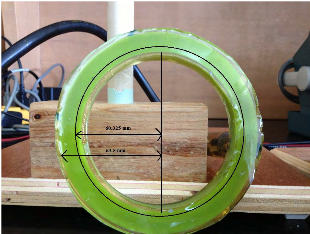
Figure 11. Urethane potted coil placed next to its wooden mounting stand.
