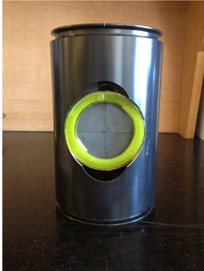
Figure 29. The receiving coil and ferrite backing plate inside of the AUV hull.
