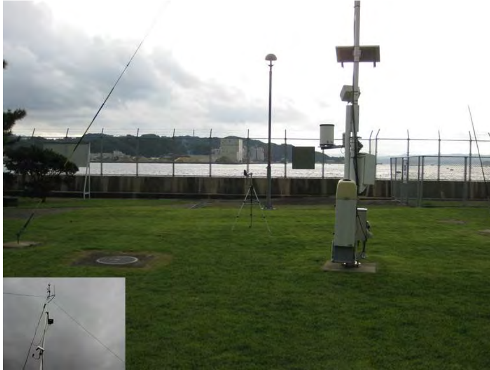
Figure 12. CFAS Vaisala installation with the top of mast indicated in the inset. View is toward the S from the approximate same location as Figures 6–10. Note that the sensor has the least obstructions from SE to the NNW. A small picnic structure is immediately to the N with low buildings and trees within ~50 m from NNE to SSE.
