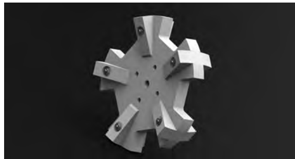
Figure 2.2: DARC Whieg design printed by a three-dimensional printer.
