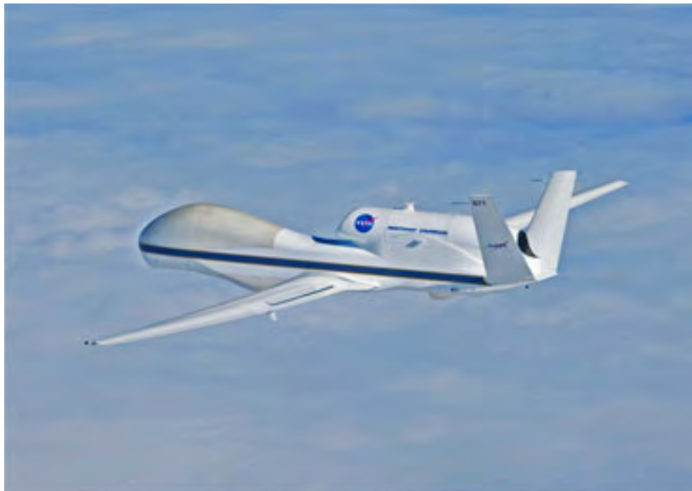
Figure 9. The NASA Global Hawk unmanned aircraft system (UAS) is capable of flight altitudes up to 65,000 feet and flight durations of up to 30 hours. An ideal platforms for investigations of hurricanes, the Hurricane and Severe Storm Sentinel (HS3) mission has utilized two Global Hawks, one with an instrument suite geared toward measurement of the environment and the other with instruments suited to inner-core structure and processes (from National Aeronautics and Space Administration 2011)
