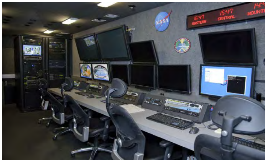
Figure 22. The interior of the NASA Global Hawk Mobile Operations Facility outfitted for operation of the Global Hawks from locations other than NASA's Dryden Flight Research Center in California. This ground control station also allows for operation of two Global Hawks simultaneously (from NASA/Tony Landis 2010. URL: http://www.nasa.gov/mission_pages/hurricanes/missions/hs3/news/pilot-challenges.html )
