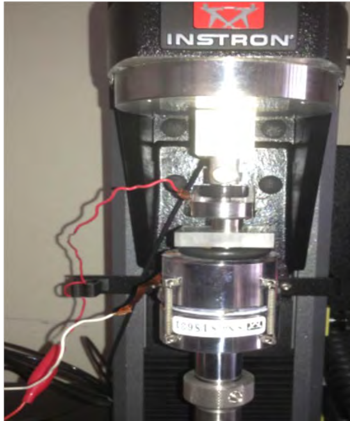
Figure 11. CFF Resistance . CFF samples were placed in the Instron such that each side of the sample was firmly in contact with copper tape attached to the Instron anvils. Measurement showed the only significant resistance was in the CFF.
