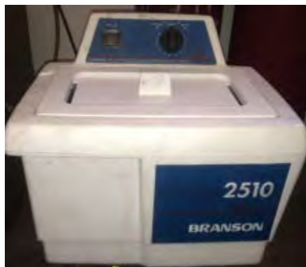
Figure 5. Catalyst Mixing. Branson 2510 sonicator utilized to mix nickel catalyst in water.
