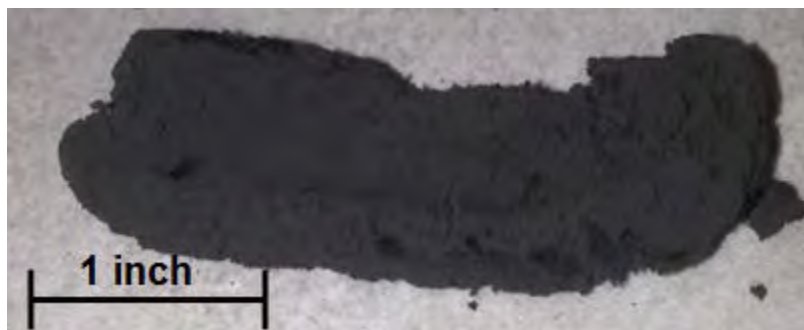
Figure 17. Carbon fiber foam grown on pure palladium. Successful shape with very little crumbling as shown.
