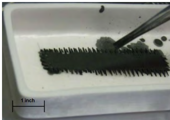
Figure 4. Carbon Mat. The process of adding nickel catalyst solution by pipette to carbon mat ( \sim 2\frac{1}{4} \times \frac{1}{2} inch) is shown.
