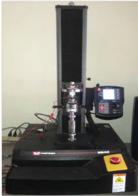
Figure 7. Mechanical Testing Apparatus: An INSTRON 5942 Compression/Tension tester (shown) was used in all transient and dynamic stress/strain tests of CFF samples.
