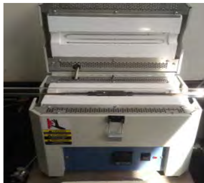
Figure 3. Furnace. For all CFF growth, the mold pictured in Figure 1 was filled with catalyst then set horizontally in an 18'' x 2'' diameter Lindberg/Blue Mini-Mite furnace (shown).
