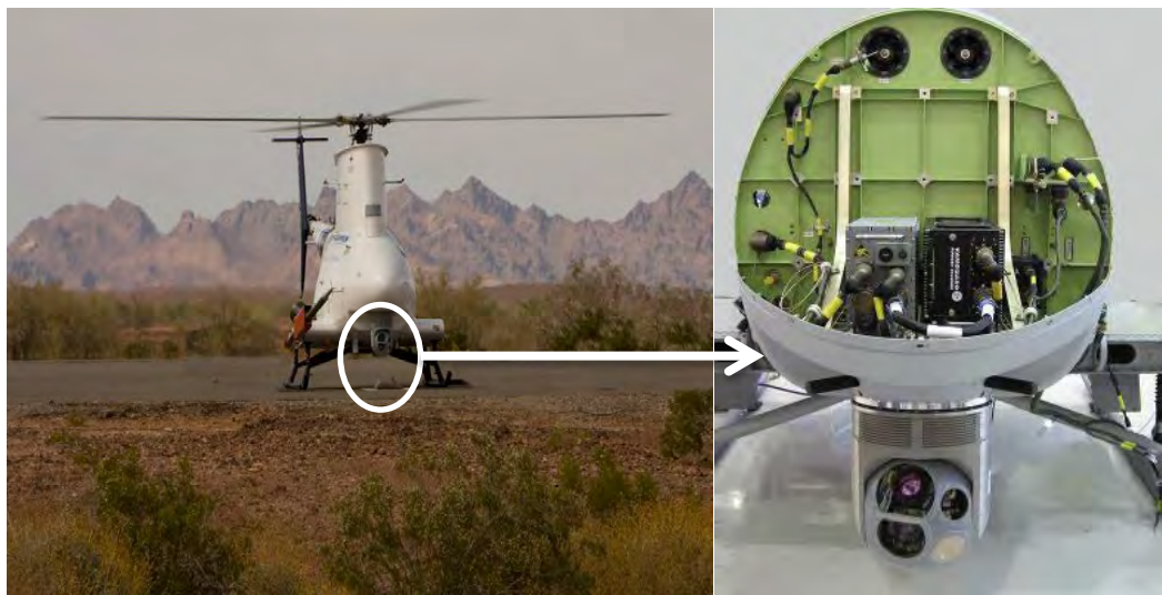
Figure 2. VTUAV with the COBRA sensor
