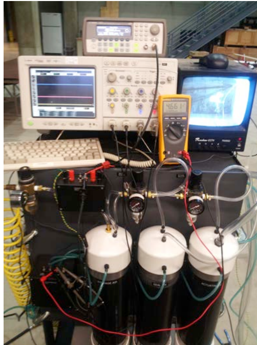
Figure 19. Test apparatus used for bench testing, submerged testing, and qualitative data collection. The monitor in the upper-right portion displays the video feed from a submerged camera, giving an unobstructed view of bubbles emerging from the nozzle and rising to the surface.
