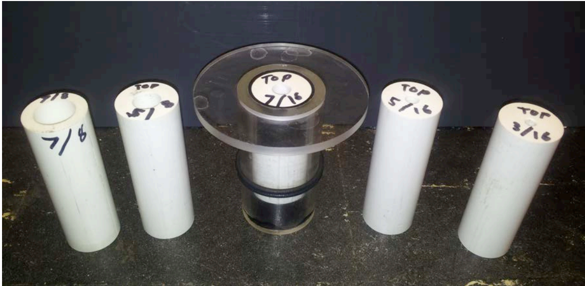
Figure 6. PVC inserts used in test model modification. The 7/16^{\text{th}} in. orifice is fitted into the test sleeve. The remaining inserts from left to right are 7/8 in., 5/8 in., 5/16 in., and 3/16 - in. diameter nozzles.
