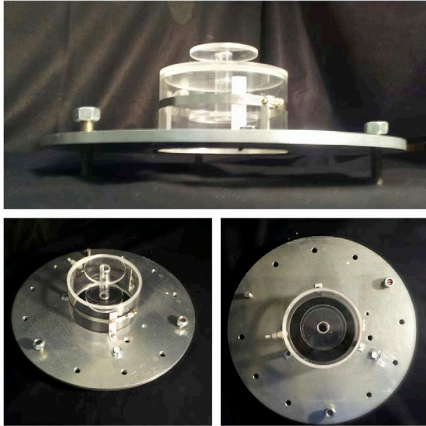
Figure 5. Assembled test model on weighted base plate, 1 in. diameter orifice installed. The lower images also show the orientation of the leveling screws and the fisheye-level bubble.
