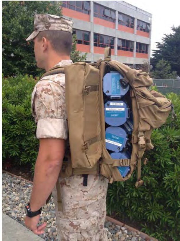
Figure 36. Side View of Nodes in Load-Bearing Pack
