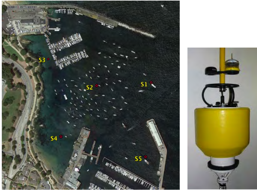
Figure 7.1: The annotated positions in the image ( S_1, S_2, S_3, S_4, S_5 ) are the locations of the gateway buoy for the first two rounds of testing (August 2011 and July 2012). For each dataset, the buoy (shown on the right-hand side) was placed at one of the locations and signal statistics were collected using this buoy as the source of a message packet where the destination was from a boat maneuvering around the harbor.
