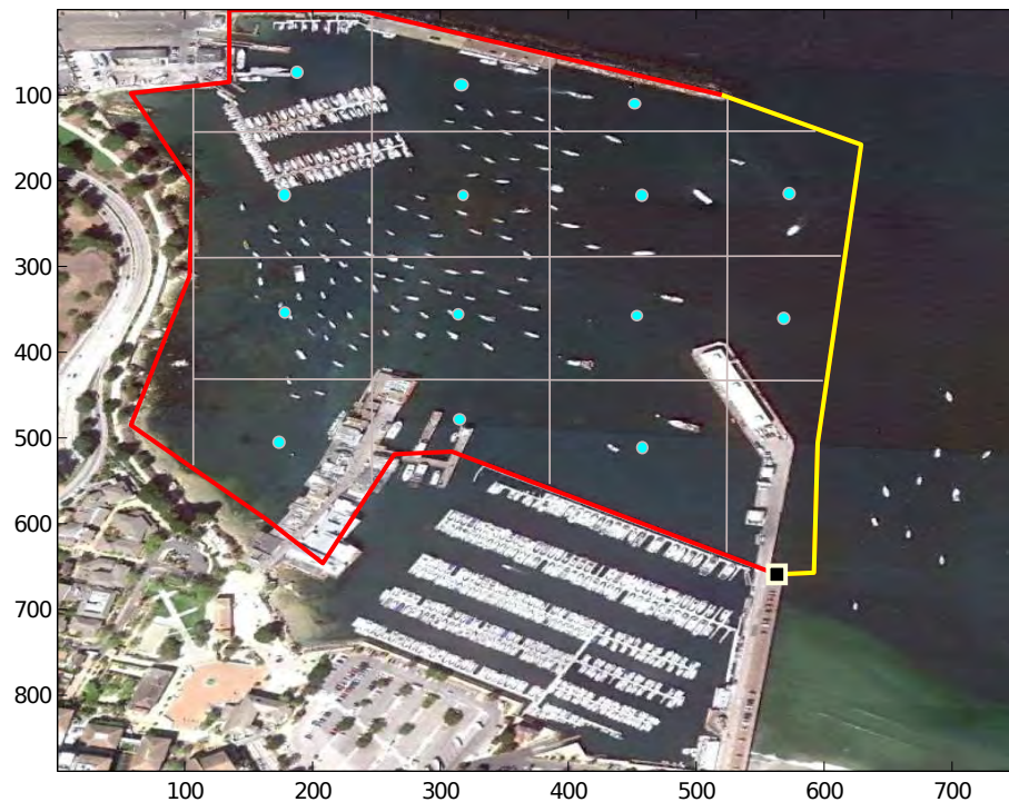
Figure 8.2: The above graphic displays an overlay that represents a visual depiction of a Global Connectivity Map. The red and yellow borders form the permeable and impermeable boundaries for an undersea GCM. The impermeable boundaries are in red and are examples of where no communication is possible outside the boundary. The permeable boundaries in yellow are examples where communication is possible outside the boundary. The gray grid represents the resolution of the map such that the goal of the estimation process to produce an LCM that is centered on the grid cell (in light blue).
