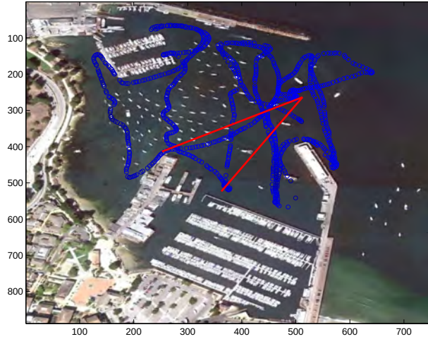
Figure 9.2: The graphic depicts the locations of acoustic signal strength measurements (in blue) from Monterey Harbor and the boundaries of the bearing window (in red) from 165 to 195 degrees where the points within the boundaries are used to estimate the random function.
