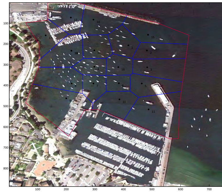
Figure 11.10: A voronoi partition with the static buoy positions acting as the control points of the partition
