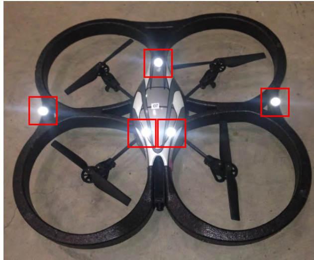
Figure 2.2: Top-down view of the Parrot AR.Drone, IR markers outlined in red for emphasis
