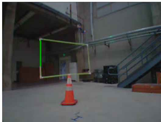
Figure 4.10: A frame of the video is analyzed using the target detection software with the skeletonize function enabled. Despite the strong edge signals, detection using the skeleton function was sporadic and inconclusive. Shown here, only partial positive detection of one side.
