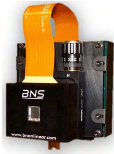
Figure 4. Spatial light modulator manufactured by Boulder Non-Linear Systems used in the experimental set-up.
