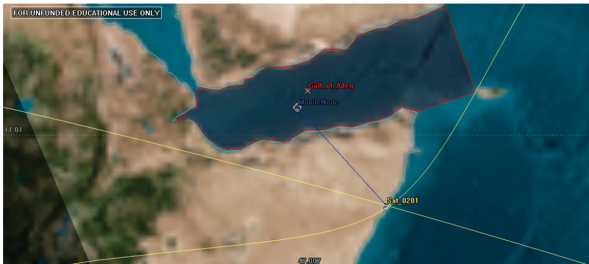
Figure 5. STK 2D graphic showing access between a satellite and the mobile node.
