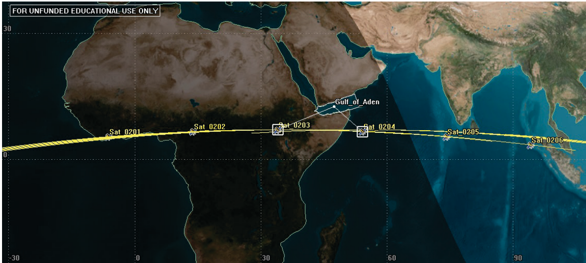
Figure 7. Ground track for inclination of 7^\circ with simultaneous access for two satellites.
