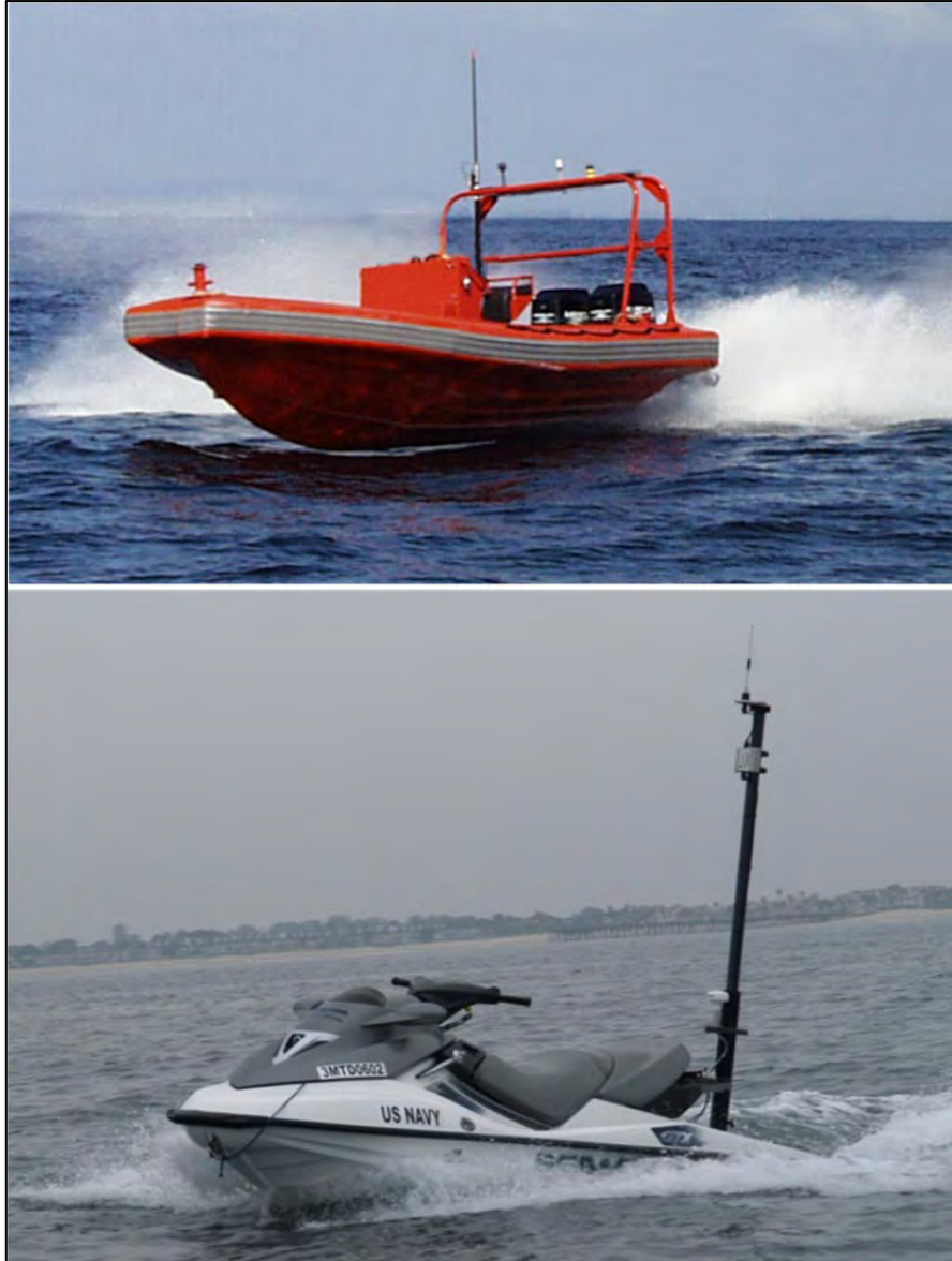
Figure 5. High speed maneuverable surface target (top), ship deployable surface target—Jet Ski (bottom), from [3].
