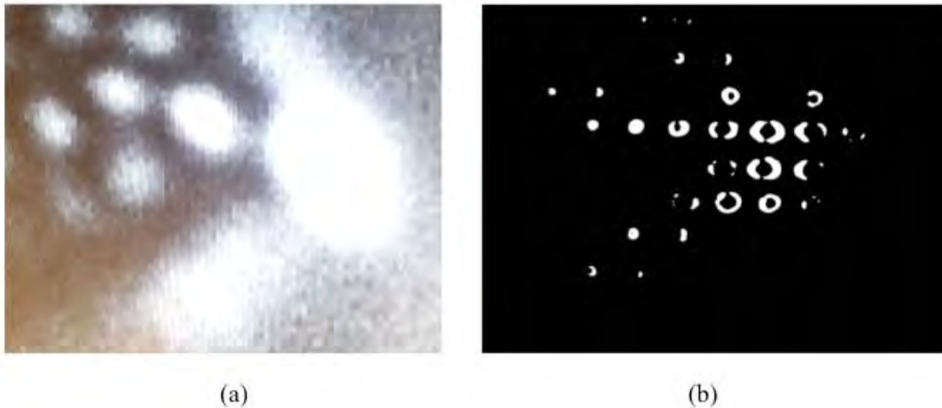
Figure 20. Imaging of QCL beam. The diffraction pattern is due to far field interference caused by the facets of the QCL laser. The QCL beam is adjusted to give a ‘mushroom’ shape in order to be imaged on the MEMS THz detector. (a) Image obtained using a commercial IR microbolometer camera. (b) Image obtained using MEMS THz detector with background subtraction. It can be observed that, due to the larger pitch size of the MEMS THz FPA as compared to the microbolometer FPA, it cannot resolve the finer details of the QCL beam.
