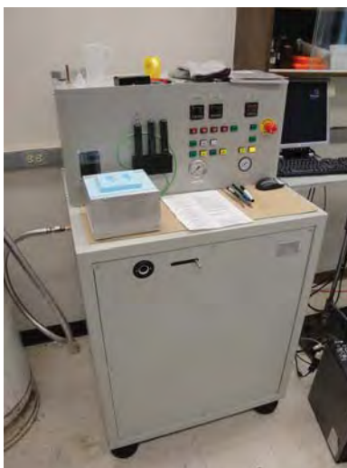
Figure 6.1: BalTec HPM 010 High Pressure Freezer.
