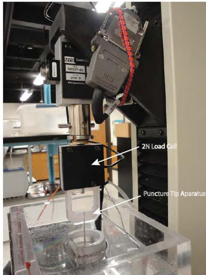
Figure 4.1: 2N Load Cell and Puncture Tip Apparatus Attached to MTS Insight II.
