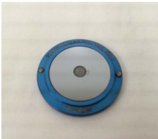
Figure 5. Zero Background XRD Sample Holder
