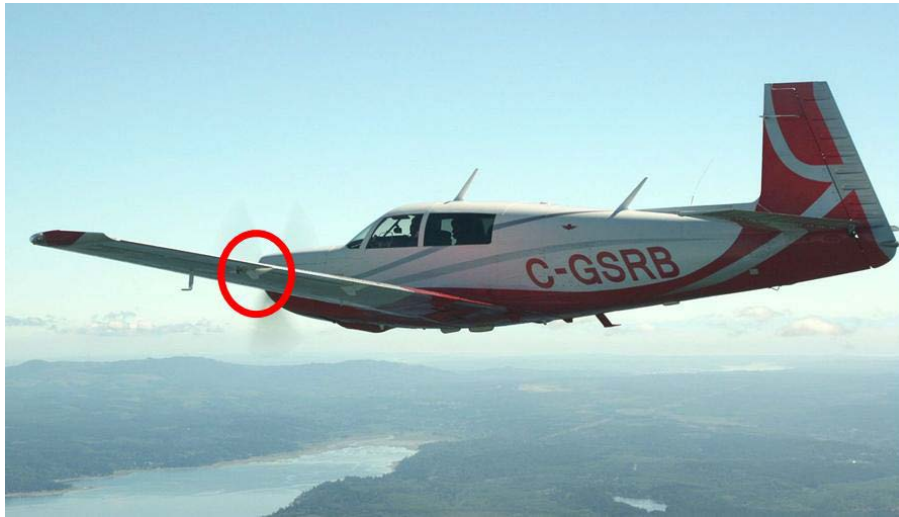
Figure 4. Example of proper sight picture in formation flight with the left wing crossing the front tip of the aircraft (from Mooney Caravan, Mooney Caravan Formation Guide , Rev. 3, Feb. 2013, p. 23).
