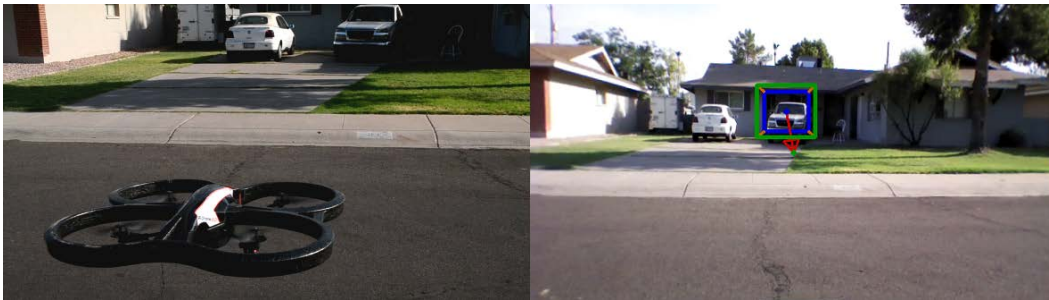
Figure 2. The Parrot AR Drone 2.0, which is used in ASTRIL's research to identify, track, and follow various targets. The left photograph shows the UAV, while the right photograph shows a view from its onboard camera with a box around its target. 3
