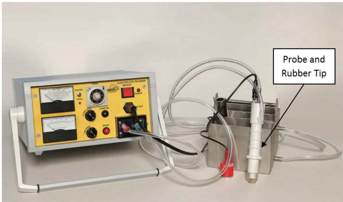
Figure 21. Proto Electrolytic Polisher Model 8818-V3 used to remove surface material for depth-resolved measurements.
