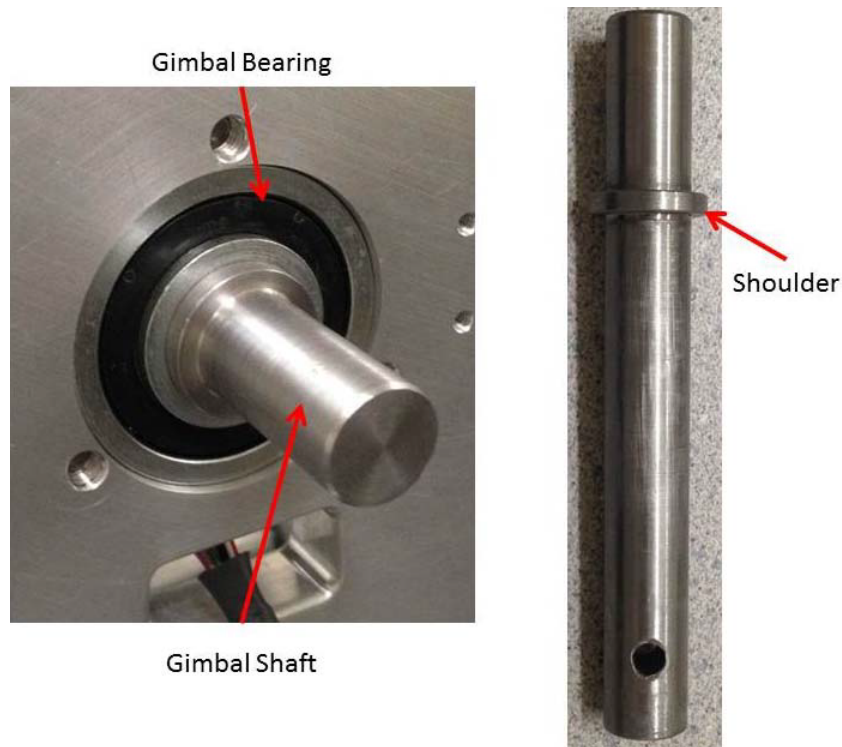
Figure 20. Bearing side gimbal shaft, (left) installed in CMG, (right) pre-installed
