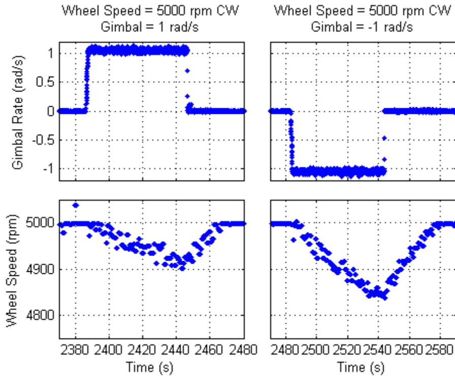
Figure 62. Momentum wheel speed with 1 rad/s gimbal rate, wheel spinning CW
