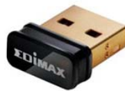
Figure 32. EDIMAX Wireless IEEE802.11b/g/n nano USB adapter, from [20]
