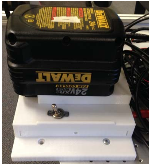
Figure 22. DEWALT 24 V battery pack and power supply block
