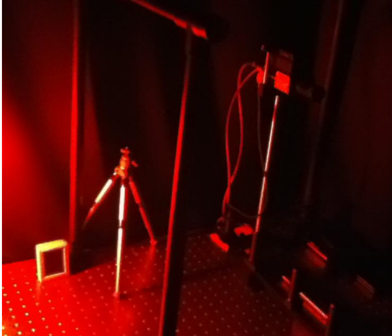
Figure 20. Hamamatsu H7421-40 PMT as part of a dark room laboratory setup used to measure the gamma scintillation response for the candidate set of crystals.
