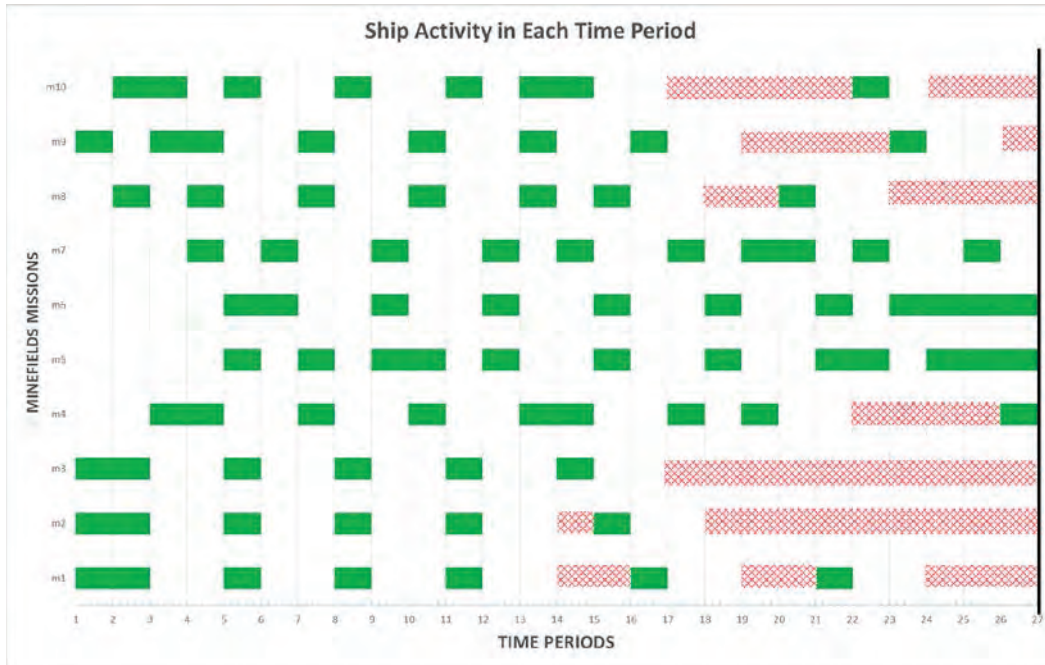
Figure 9. Chart showing ship activity throughout the phase. The solid (green) bars represent how effort is applied by the ships in each mission. In periods t1 t5, at most seven ships can be active. In periods t16 t20, when there are only two ships available, there are at most two ships working. The cross-hashed (red) bars indicate when each mission has gone idle and LOE towards mission accomplishment is degrading.
