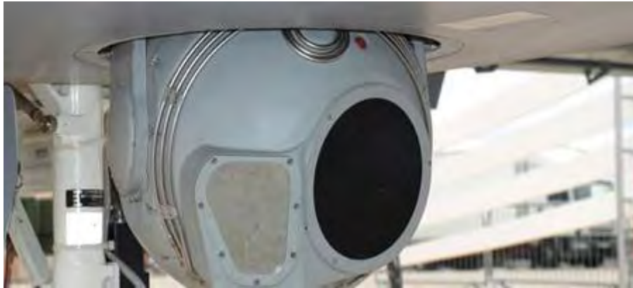
Figure 3. EO/IR payload (from Defense-Update, 2009)
