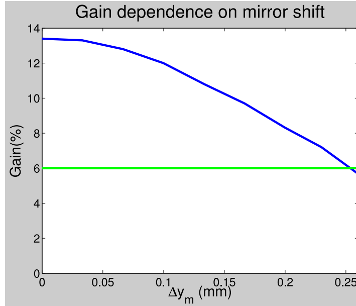
Figure 26. 4DPULSEN simulation results for weak field gain as a function of shift of one of the cavity mirrors.
