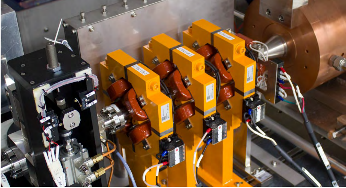
Figure 32. Quadrupole triplet for transverse beam focusing, from [23].
