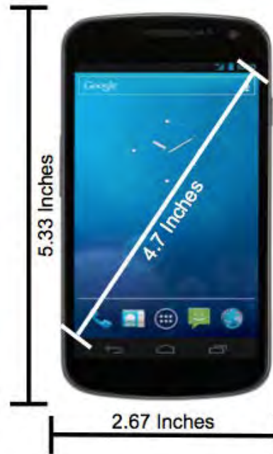
Figure 1. Samsung Galaxy Nexus Dimensions, from [31]
