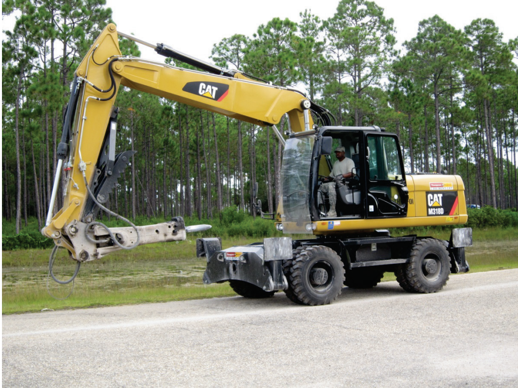
Figure 14. Caterpillar M318D excavator with H120E hammer attachment.
