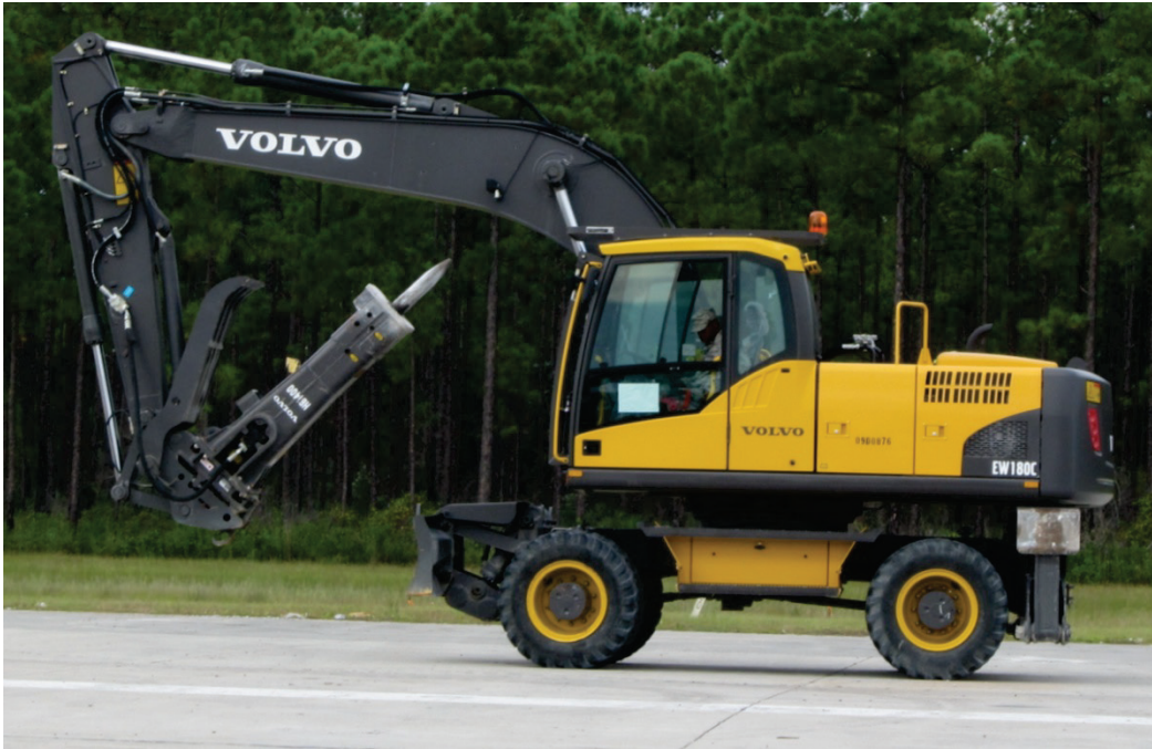
Figure 12. Volvo EW180C excavator with HB1400 hammer.
