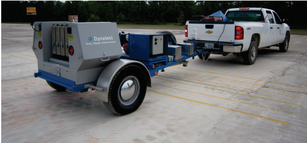
Figure 52. HWD testing on repaired crater.
