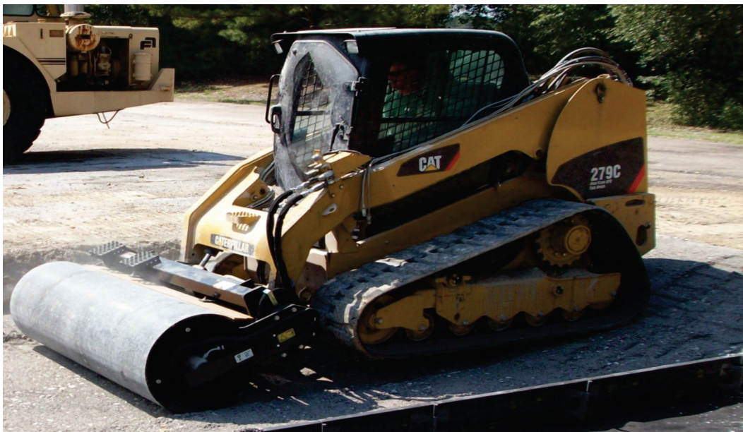
Figure 7. Caterpillar CV18B roller attached to Caterpillar 279C CTL.
