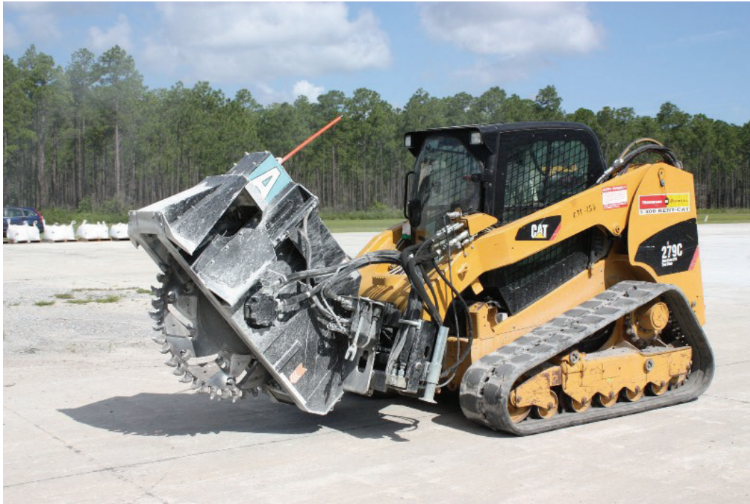
Figure 4. Tracked Caterpillar 279C CTL with SW45 wheel saw attachment.
