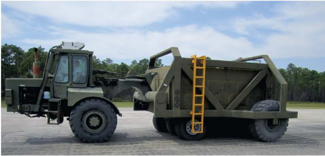
Figure 61. Trafficking with full-gear C-17 load cart.
