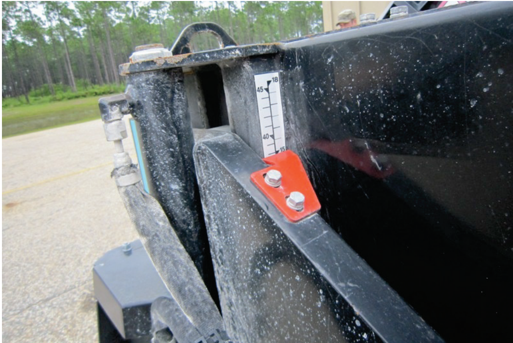
Figure 8. Ruler on top of wheel saw for lowering and raising guard according to desired cut depth.
