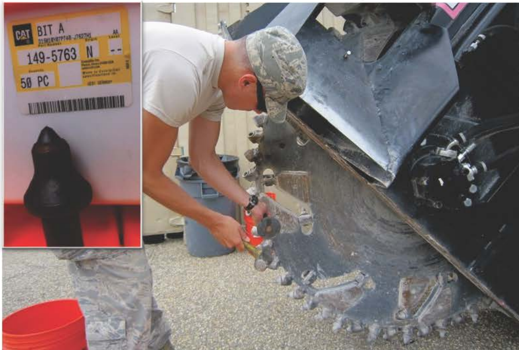
Figure 5. Replacing wheel saw teeth; inset shows close up of wheel saw teeth.
