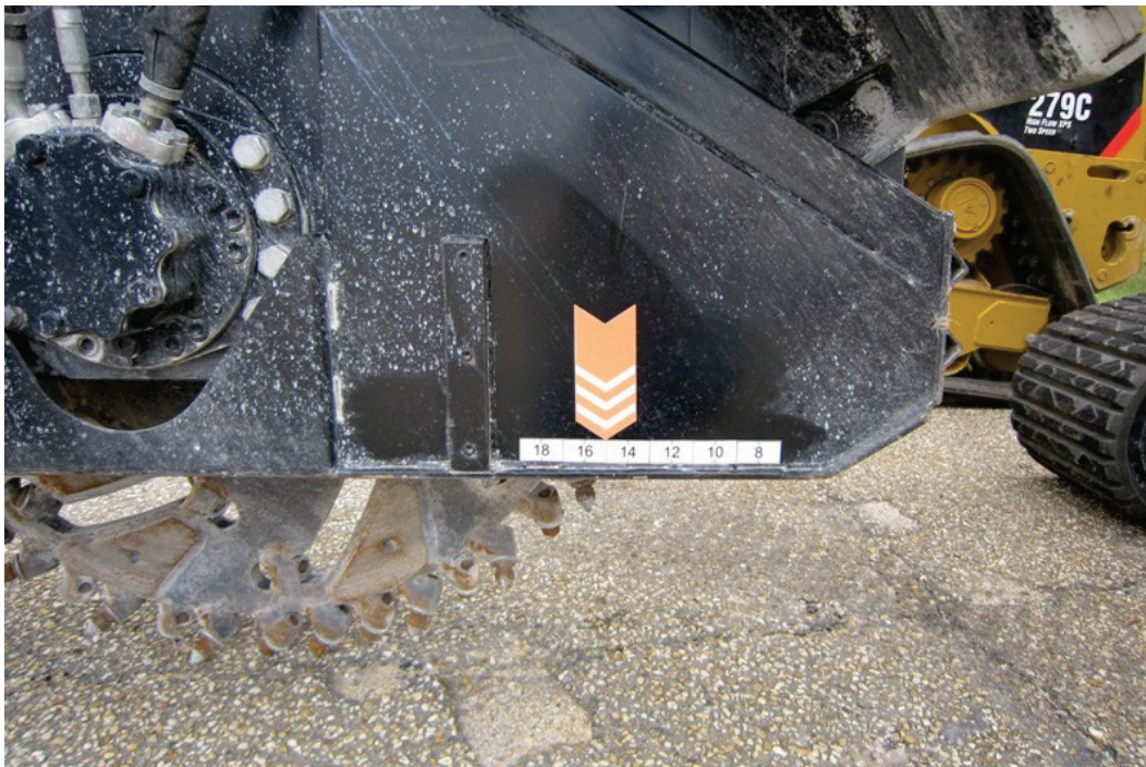
Figure 9. Ruler for lining up wheel saw according to pavement thickness or cut depth.
