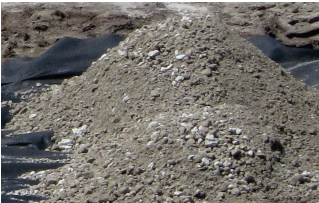
Figure 24. Crushed limestone backfill.
