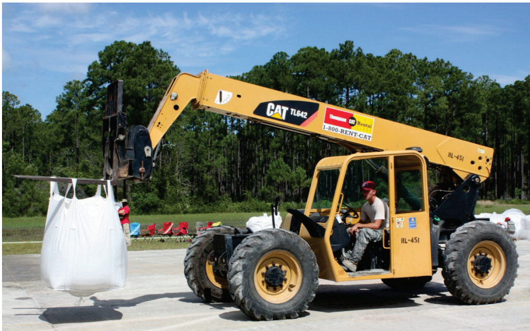
Figure 17. Caterpillar TL642 extendable-boom forklift.
