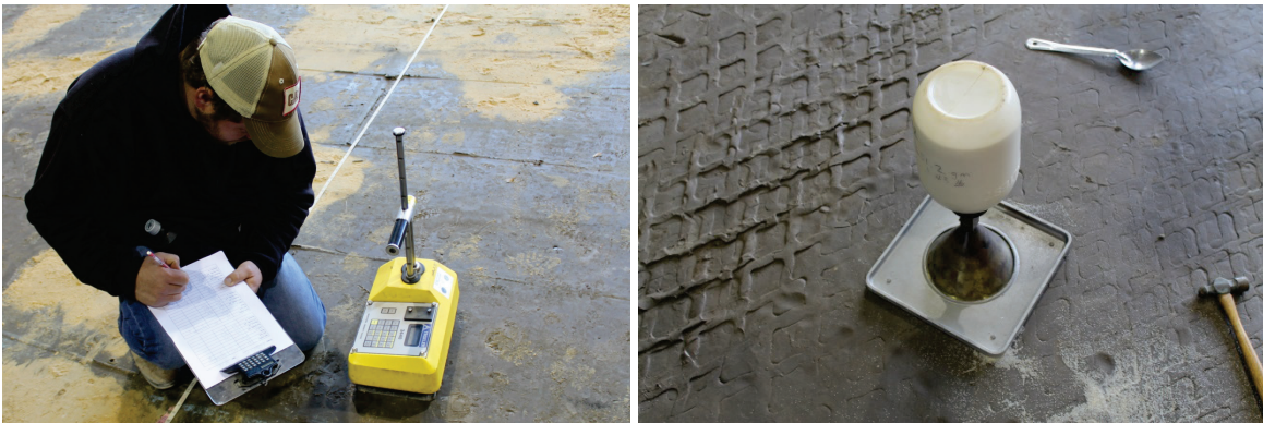
Figure 13. Nuclear gage (left) and sand cone (right) test.
