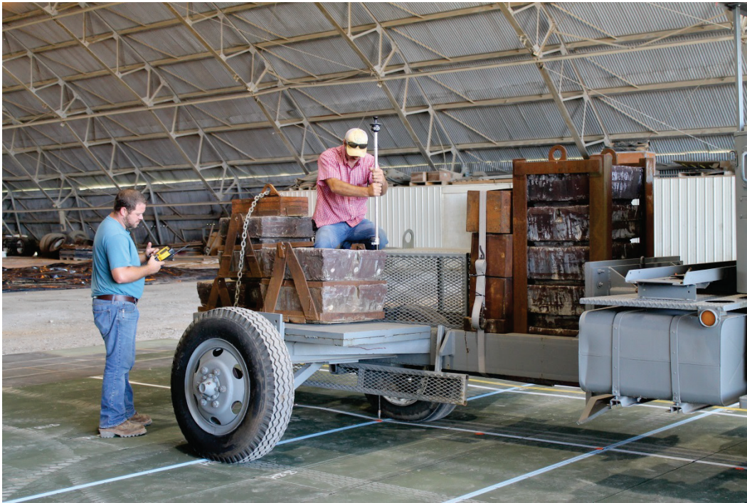
Figure 25. Elastic deflection measurement.
