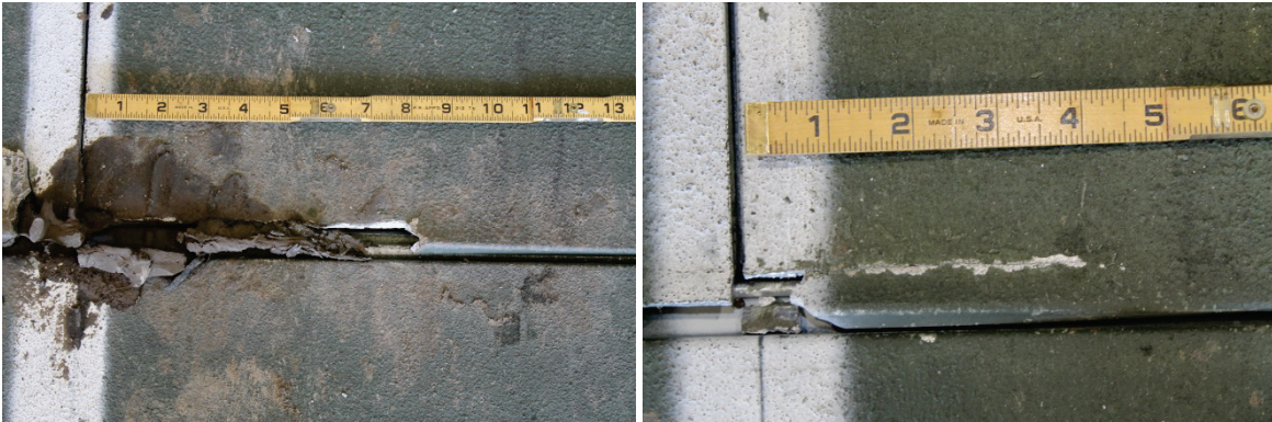
Figure 28. Top skin tear at I-7 (left) and I-34 (right).
