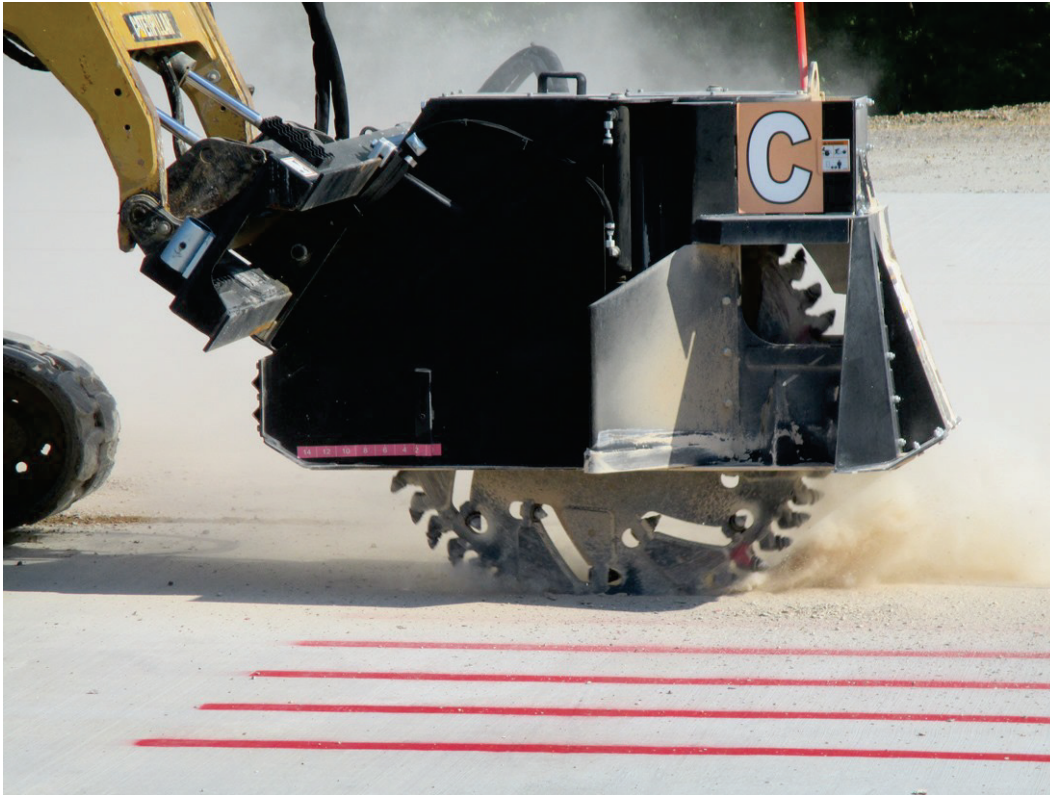
Figure 11. Caterpillar SW45 wheel saw attachment.
