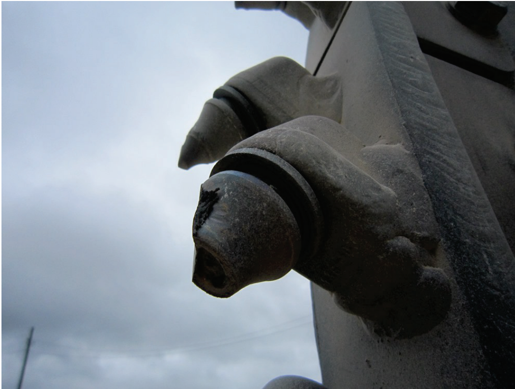
Figure 47. Sandvik F203 teeth after cutting through chert aggregate PCC.
