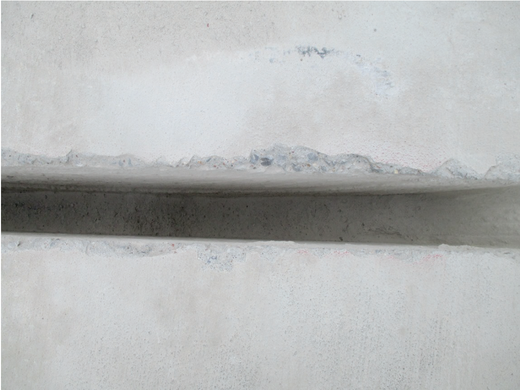
Figure 50. Spalling of limestone PCC from Kennametal RP15 teeth on CAT SW45.
