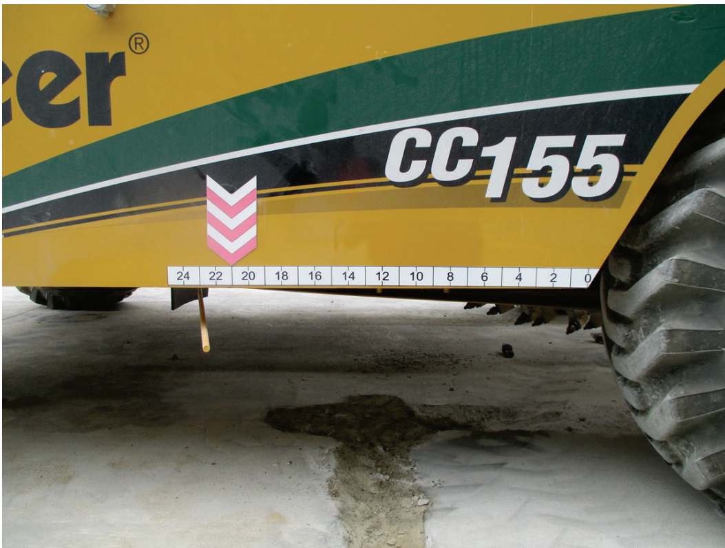
Figure 35. Ruler adhered to middle of Vermeer CC155 to aid in stopping the cut.
