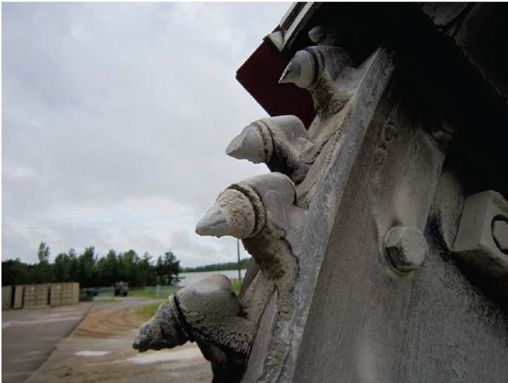
Figure 46. Sandvik F203 teeth after a wet cut through limestone aggregate PCC.
