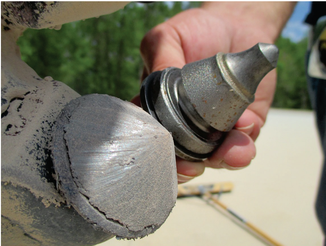
Figure 40. Short Kennametal RP15 tooth on CAT SW45 after cutting in chert PCC.
