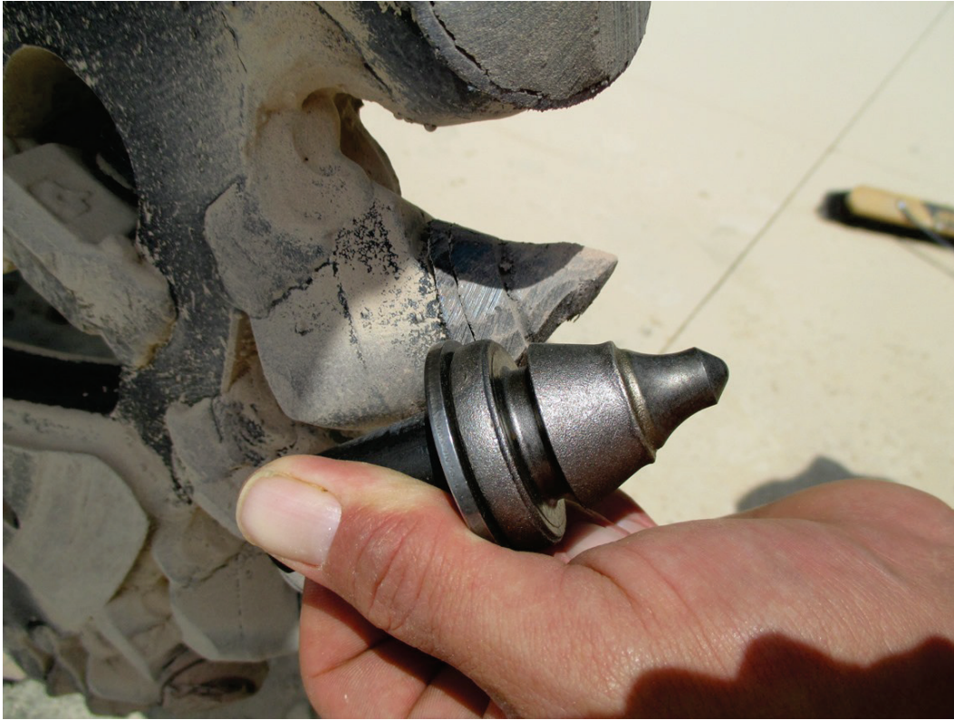
Figure 39. Worn Kennametal RP15 tooth on CAT SW45 after cutting in chert PCC.
