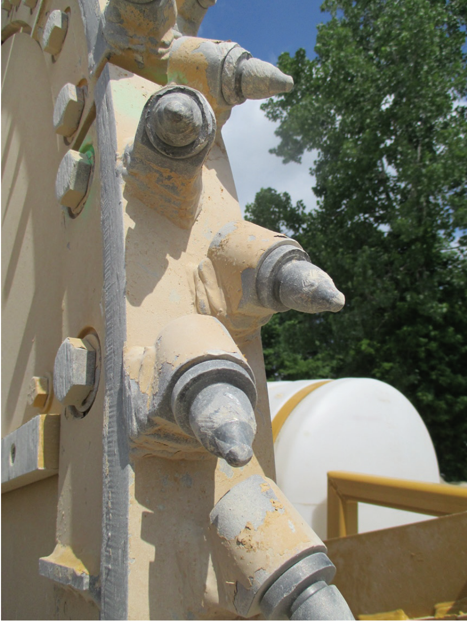
Figure 42. Kennametal SM04 teeth after cutting with Vermeer CC1531 in chert PCC.
