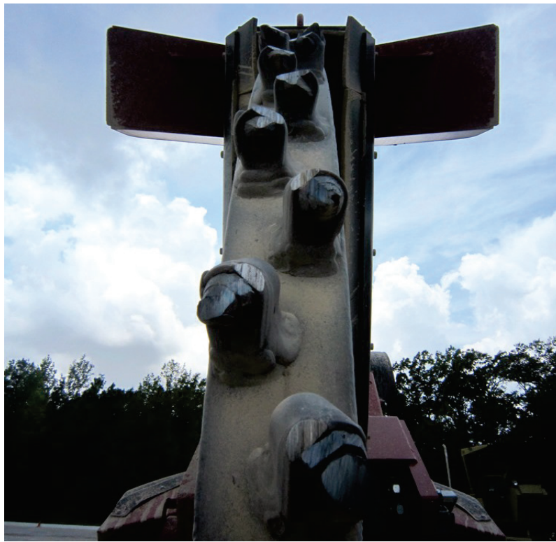
Figure 43. Kennametal SM04 teeth after cutting in chert PCC with Ditch Witch H1140 saw.
