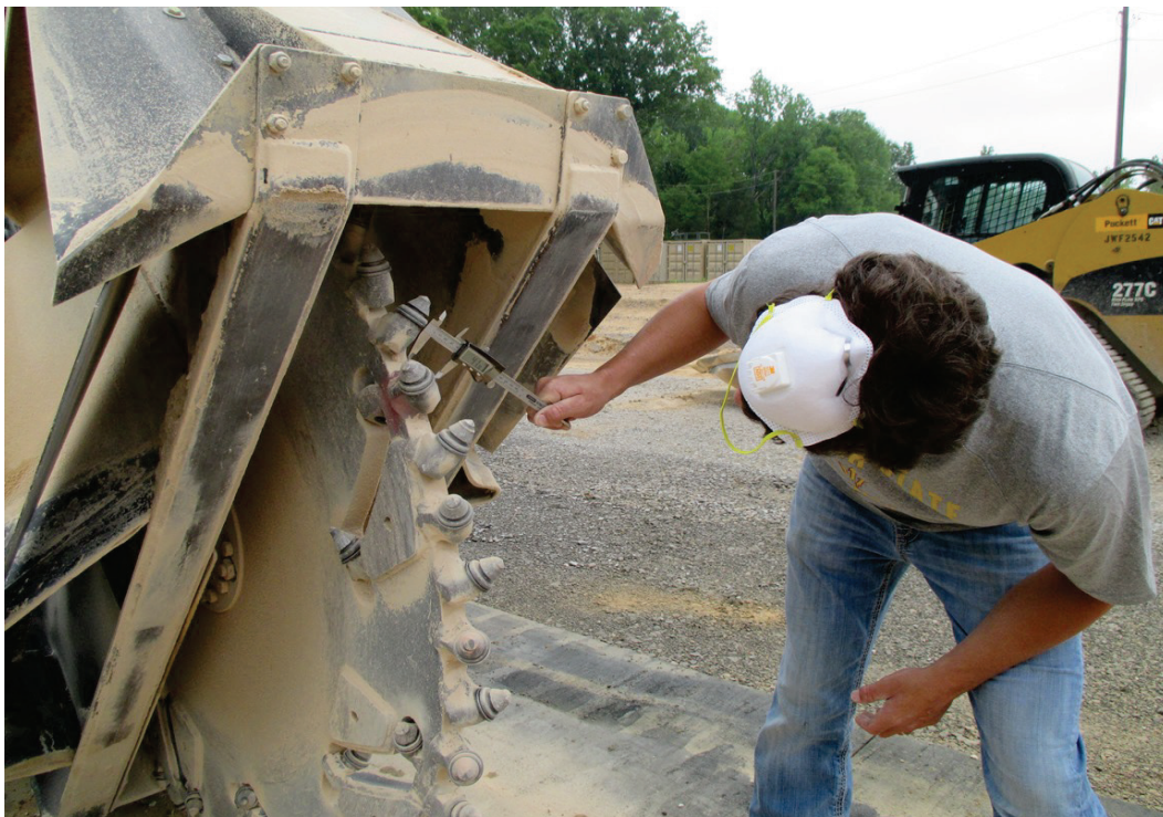
Figure 36. Measuring teeth wear using calipers.
