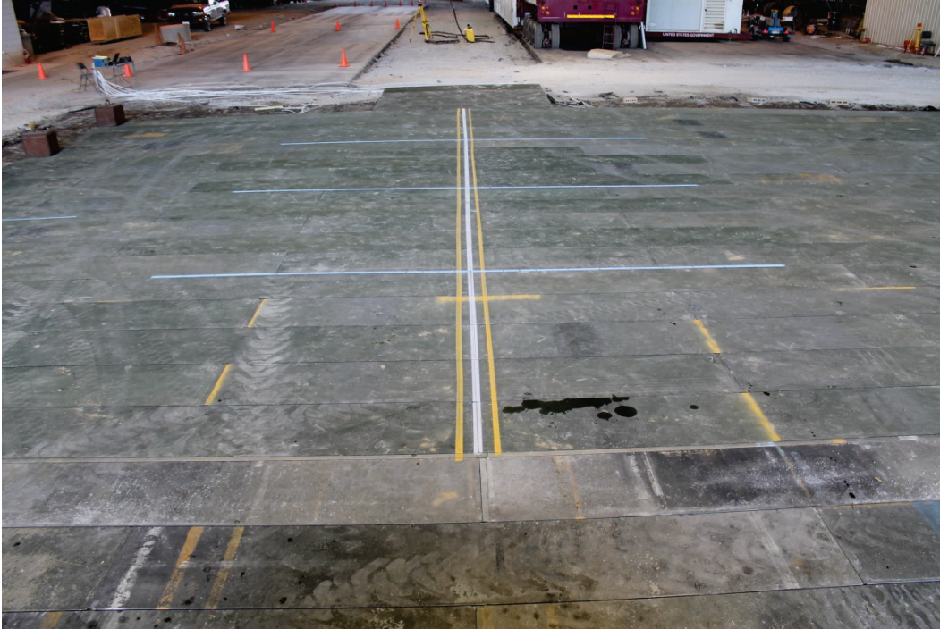
Figure 29. Brickwork pattern on voided subgrade final assembled test section.
