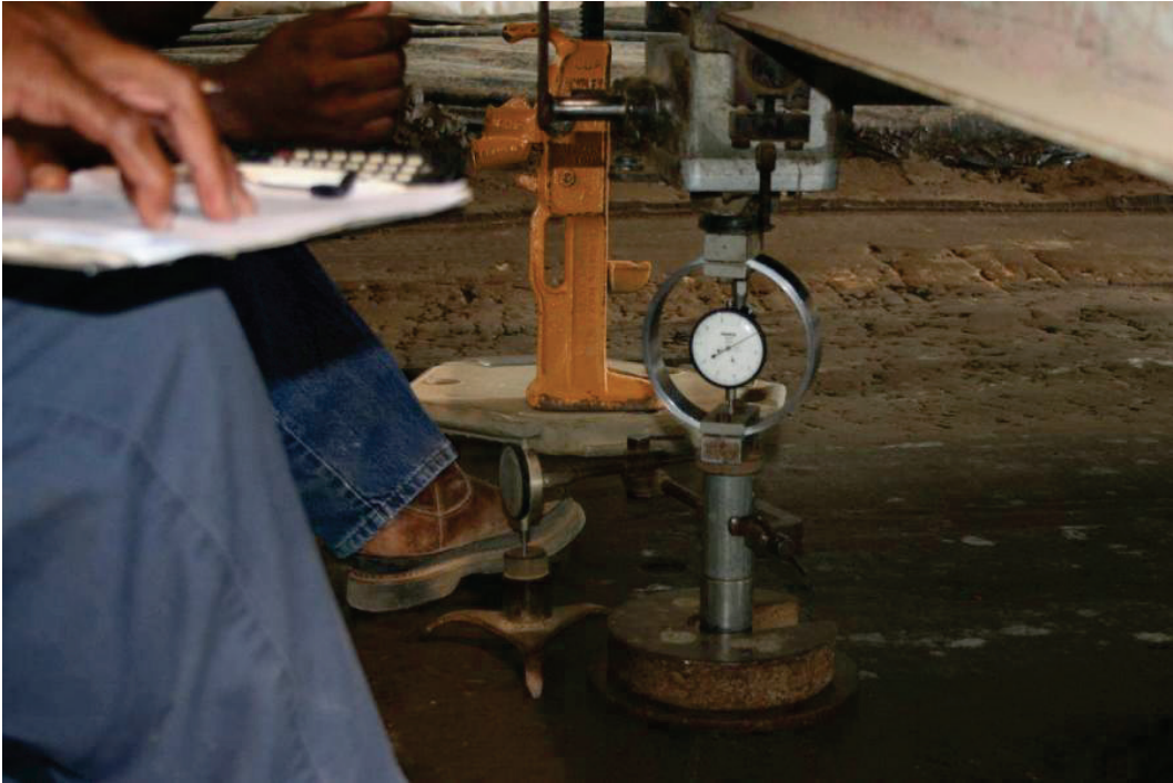
Figure 17. Field CBR test.
