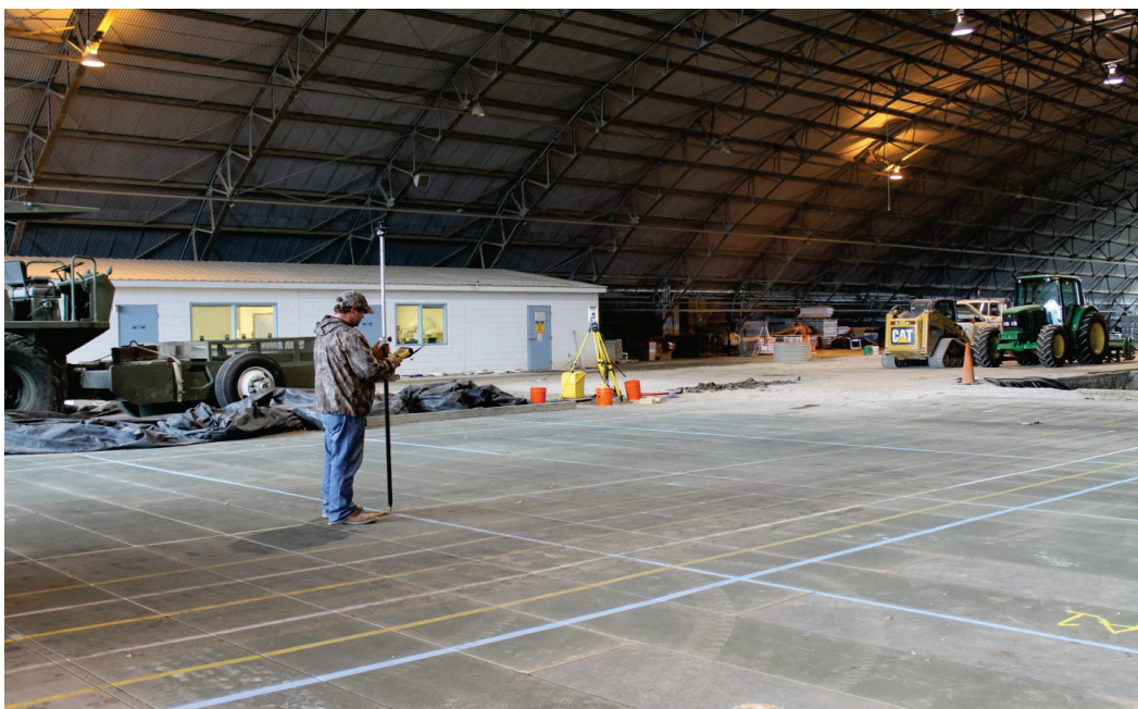
Figure 37. Surveying unloaded cross-section.
