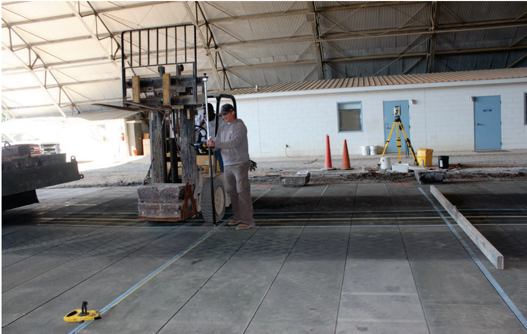
Figure 38. Surveying loaded cross-section.
