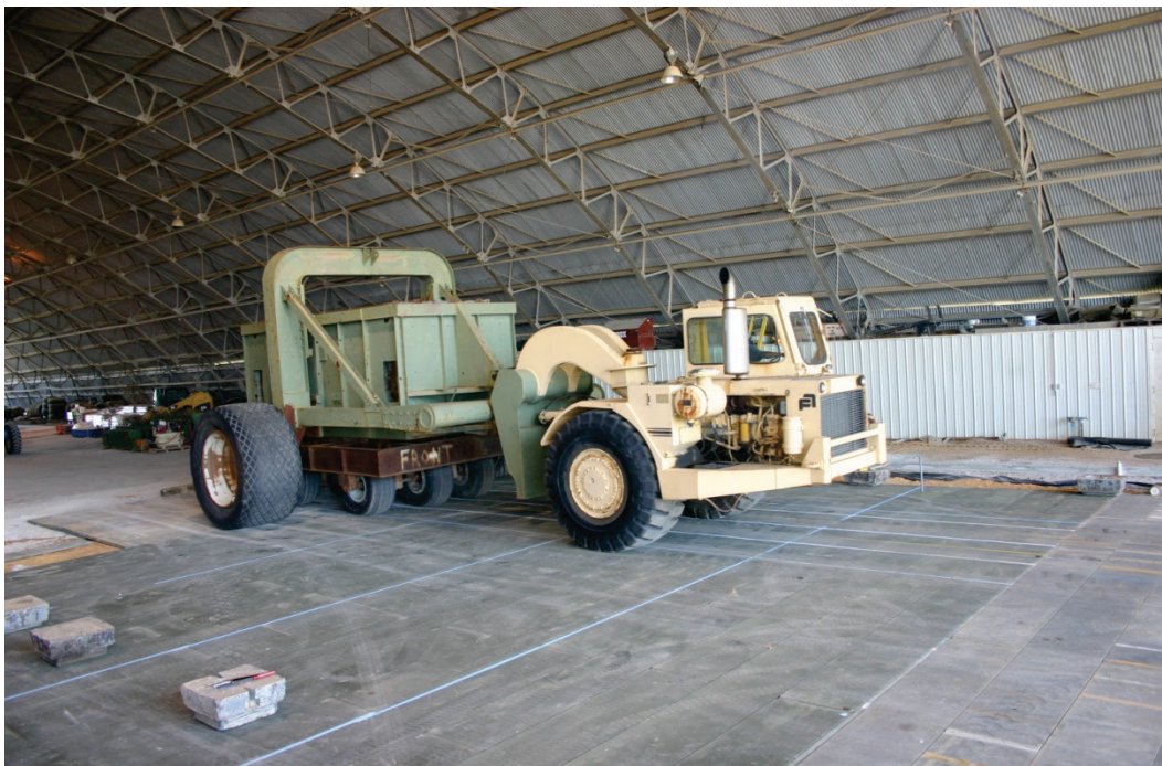
Figure 33. C-17 test load cart.
