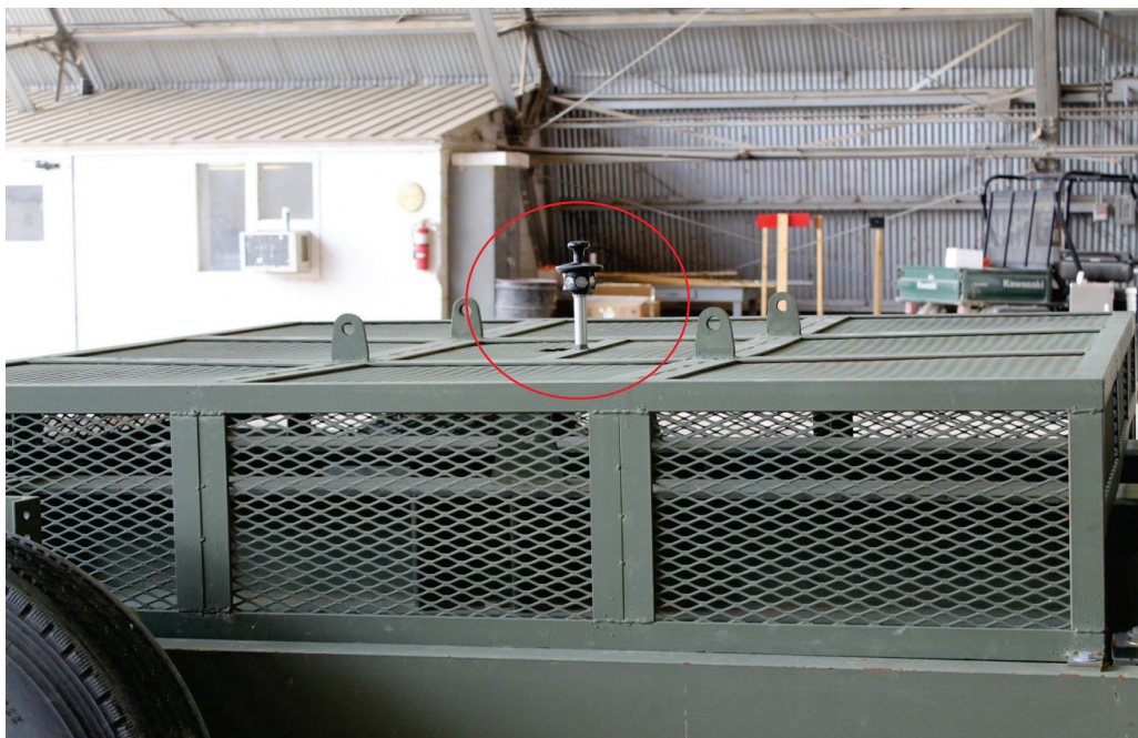
Figure 39. Prism mounted on F-15E load cart.
