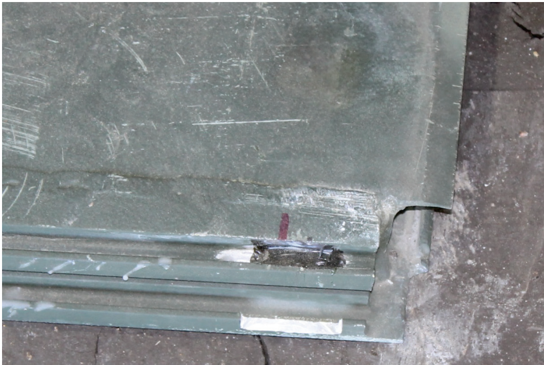
Figure 22. Typical strain gauge installation on lower overlap region.
