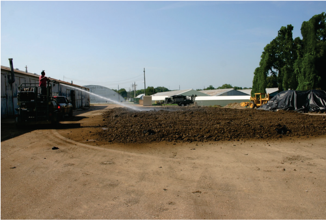
Figure 12. Addition of water to adjust moisture content.
