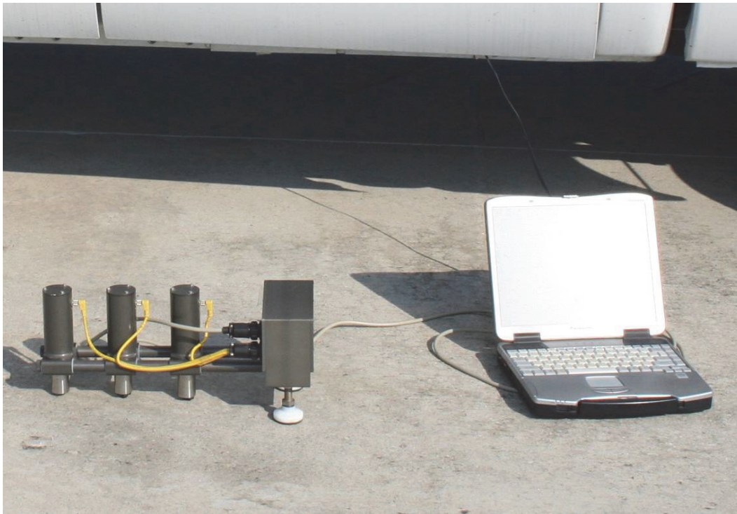
Figure 4. PSPA equipment and laptop.
