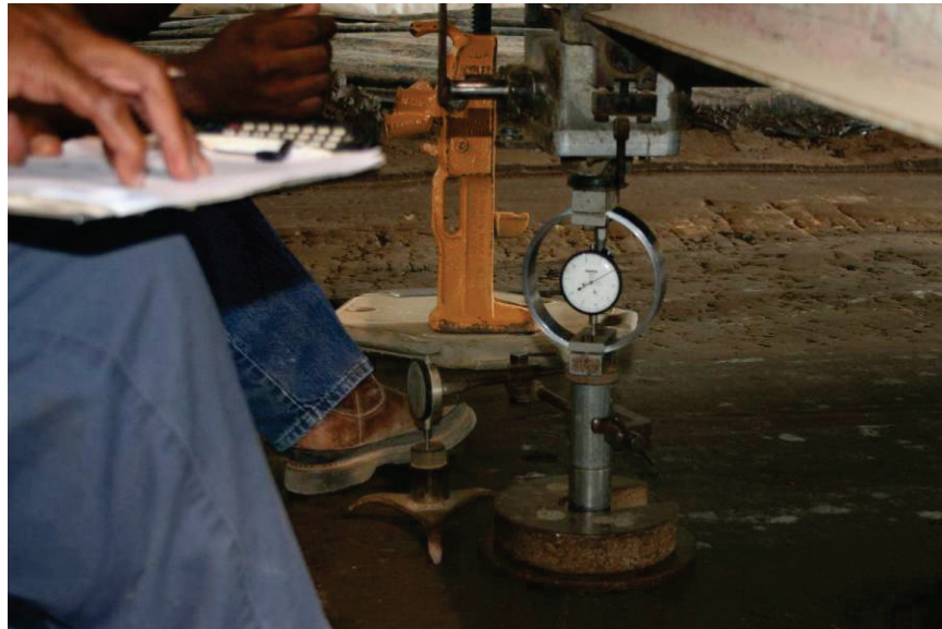
Figure 14. Field CBR test.
