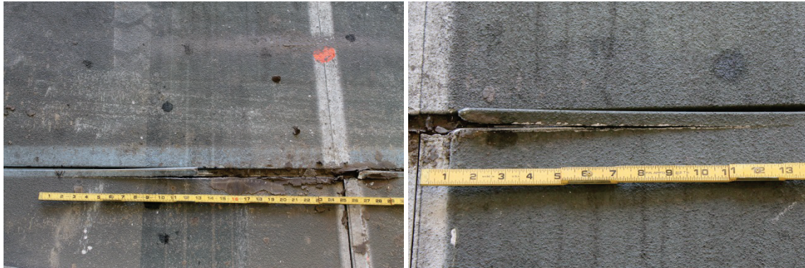
Figure 26. Top skin tear on J46 (left) and J33 (right).
