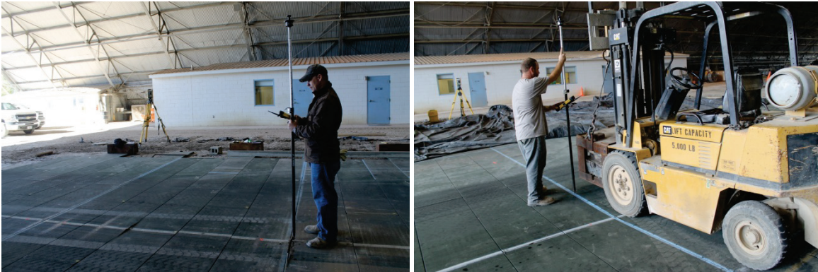
Figure 23. Surveying unloaded (left) and loaded (right) cross section.
