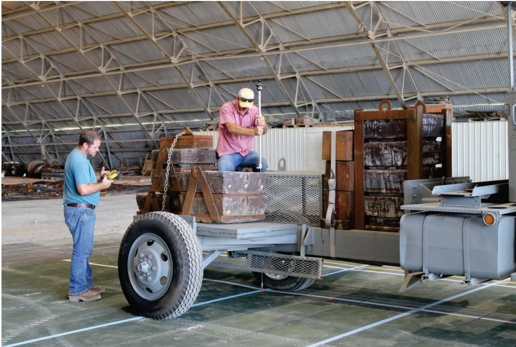
Figure 24. Elastic deflection measurement.
