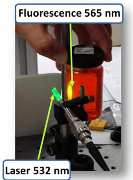
Figure 7. The 532 nm laser exciting a response from F-76 seeded with pyrromethene 597.
