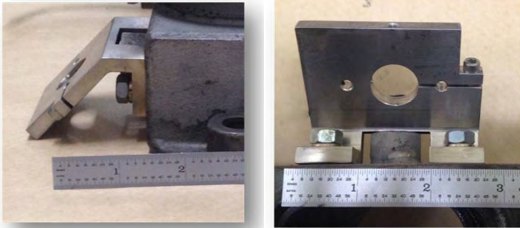
Figure 17. External instrument bracket shown mounted to a Detroit Diesel 3-53 exhaust manifold.
