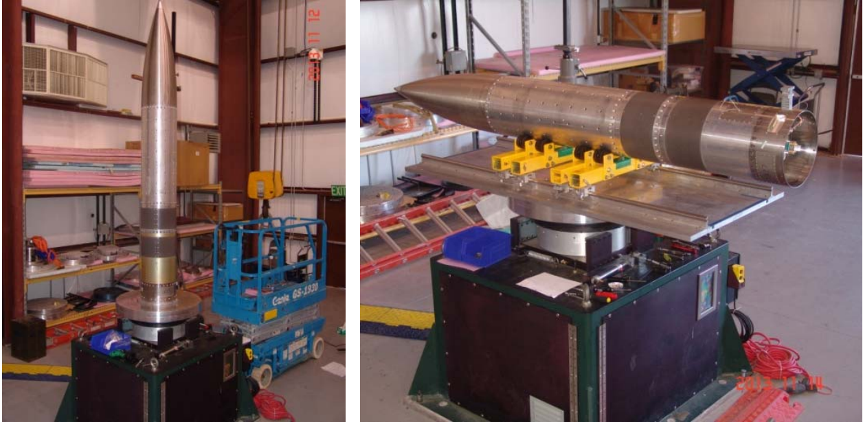
Figure 1. WSMR mass properties measurement machine.
