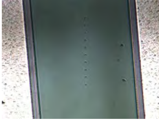
Figure 17. Ten nanoindentations of AlN film.
