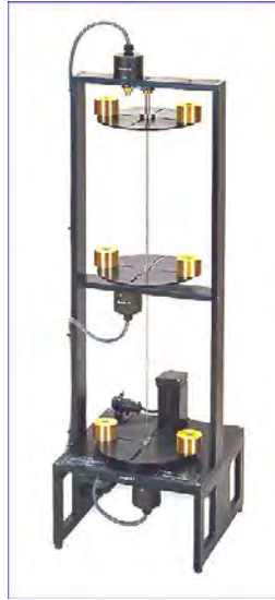
Figure 30 Torsion control plant
