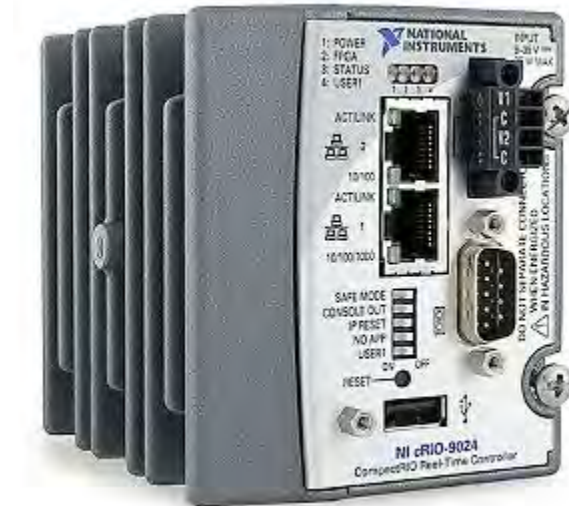
Figure 17 NI cRIO-9024 real-time controller, from [22]
