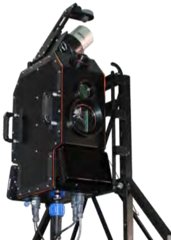
Figure 2. Contractor-developed scanning rig including GPS, long-wave infrared, near infrared and LIDAR instrumentation.
