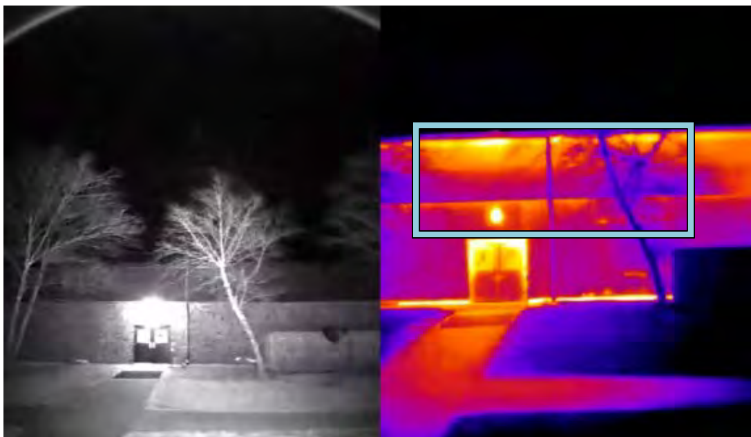
Figure D-113. NIR image (left) and thermal image (right) of Bldg 3189, Scott AFB. The top of the double doors are losing considerable energy.
