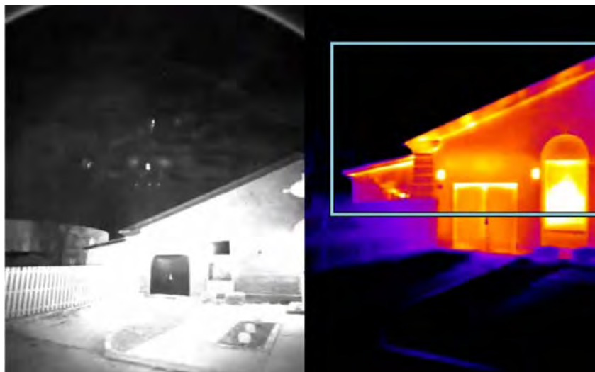
Figure D-14. NIR image (left) and thermal image (right) of Bldg 8, Scott AFB. Areas of the wall and the soffit appear to exhibit high heat loss.
