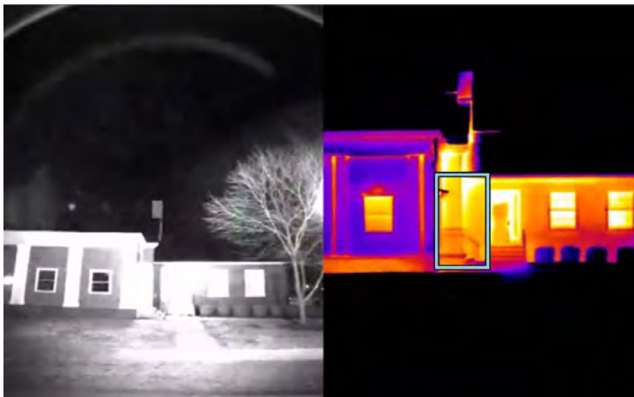
Figure D-4. NIR image (left) and thermal image (right) of Bldg 5, Scott AFB. Highly emissive door frame shown in polygon at the right.
