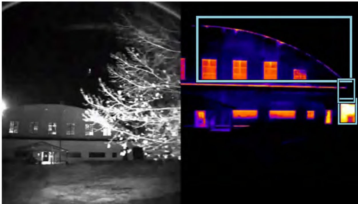
Figure D-42. NIR image (left) and thermal image (right) of Bldg 506, Scott AFB. A particularly emissive area is shown in the rectangle to the right.
