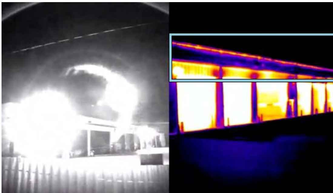
Figure D-47. NIR image (left) and thermal image (right) of Bldg 548, Scott AFB. The garage doors and soffit areas appear to be thermally inefficient.
