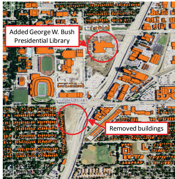
Figure 3.18. Additional edits to the building data set.
