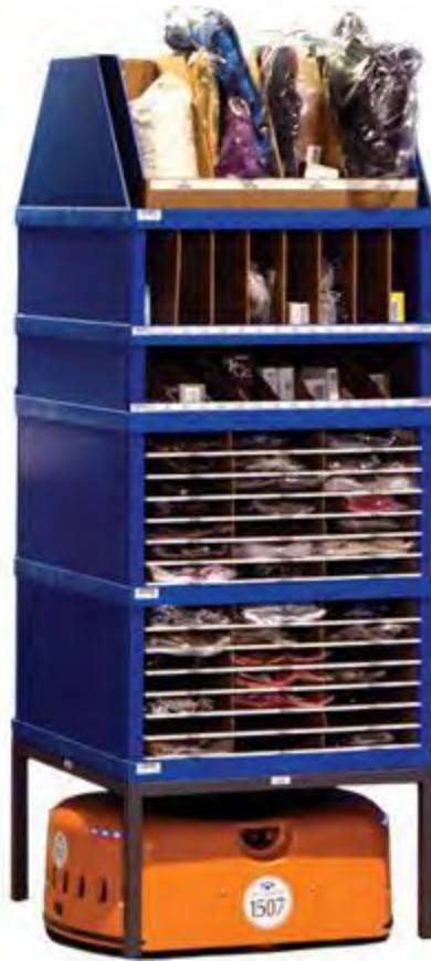
Figure 5. Kiva Robotic Drive Unit and Mobile Inventory Shelf (from Kiva, 2014)
