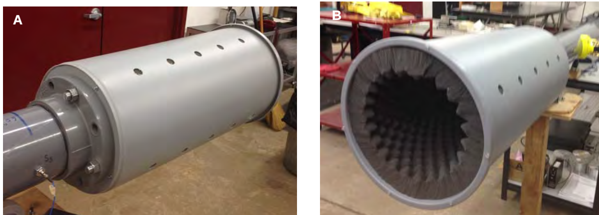
Figure 5. A sound absorption chamber was designed and installed to the end of the shock tube (A) to decrease the decibel level of the shock tube. (B) The chamber is lined with sound absorbing foam.
