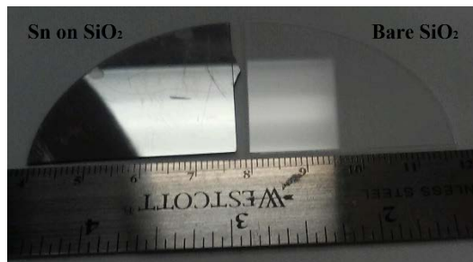
Fig. 1 Image of tin layer on \frac{1}{4} -wafer of \text{SiO}_2 (left) and bare \frac{1}{4} -wafer of \text{SiO}_2 (right)
