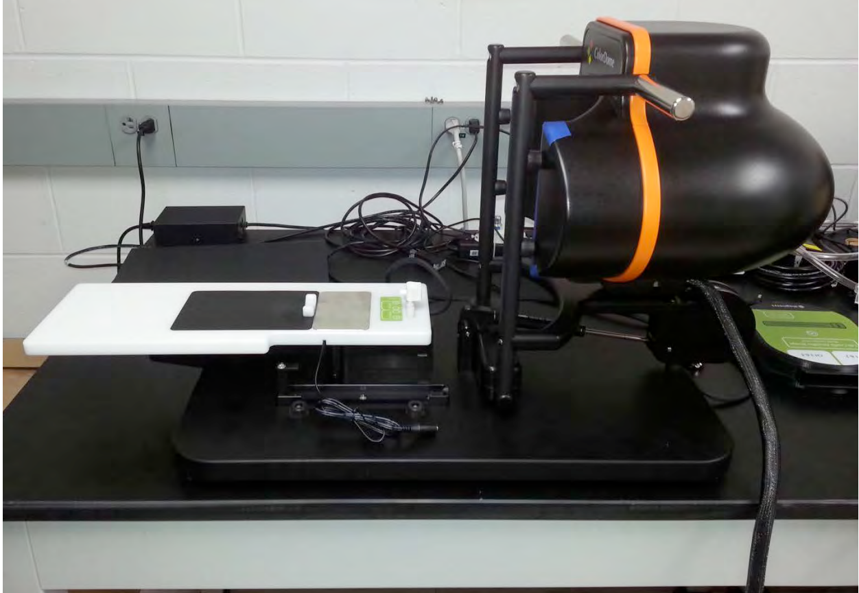
Figure 9. A look at the Diagnosys Ganzfeld bowl which provides the light stimulus to the mice. The bowl has been made to hinge into position over the mouse to provide wide field visual stimulation, in parallel to human experiments.
