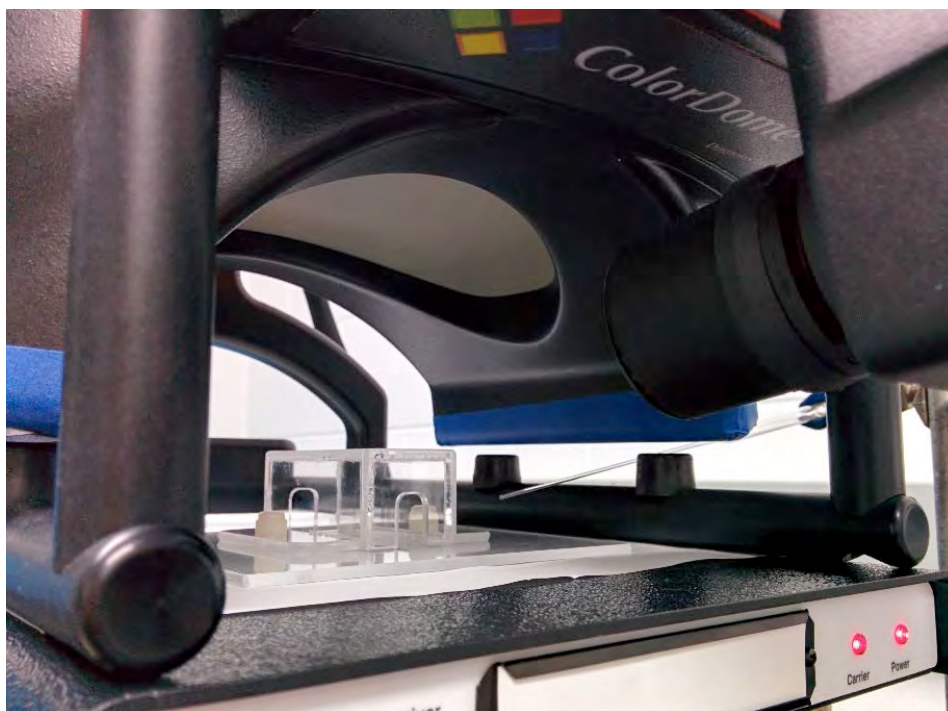
Figure 11. As part of the current testing protocol, the mice are gently restrained using a custom made acrylic box that allows video recording of blink activity with our in-house video recording system, described earlier. Light stimuli are delivered using the Diagnosys ColorDome light bowl after a dark adaptation period of 15 minutes, while the DSI plate reader below the acrylic mouse holder is used to transfer the EMG signals from the mouse wirelessly to a computer.
