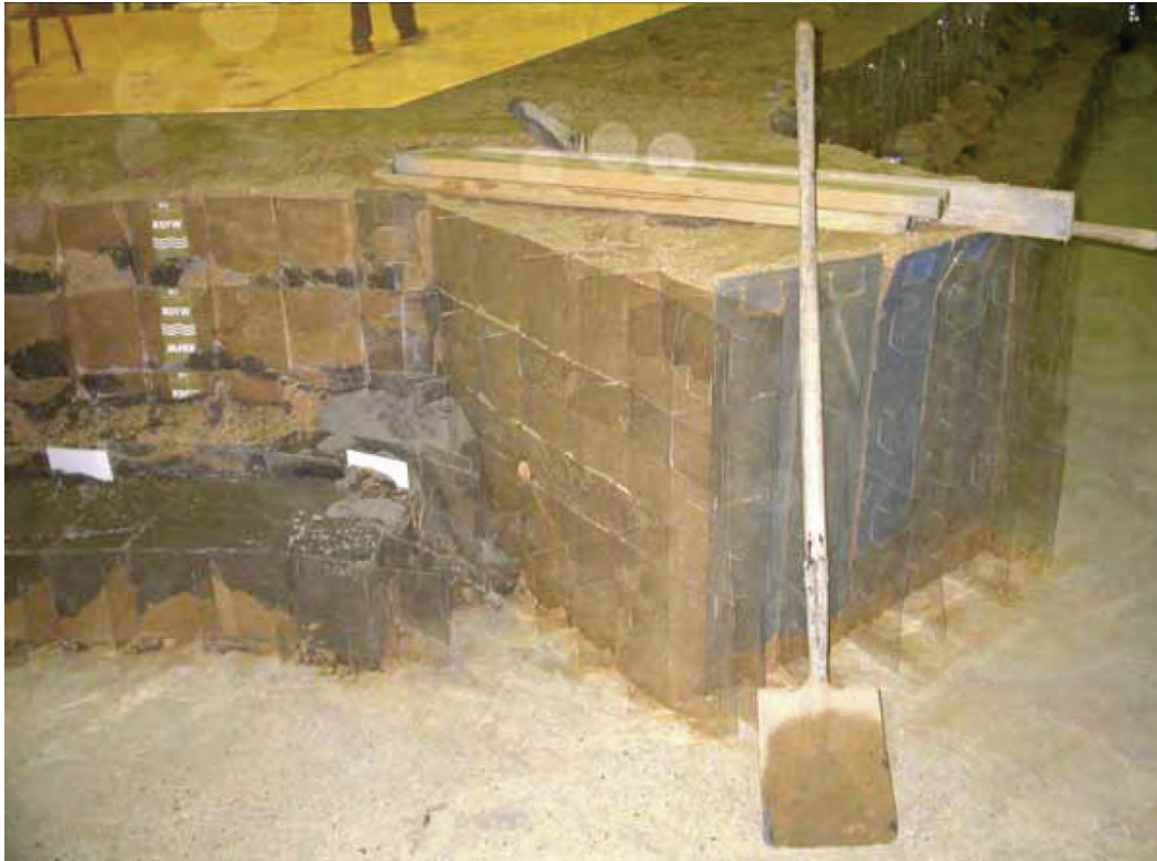
Figure 5-3. Laboratory Rapid Deployment Flood Wall (USACE 2007).
