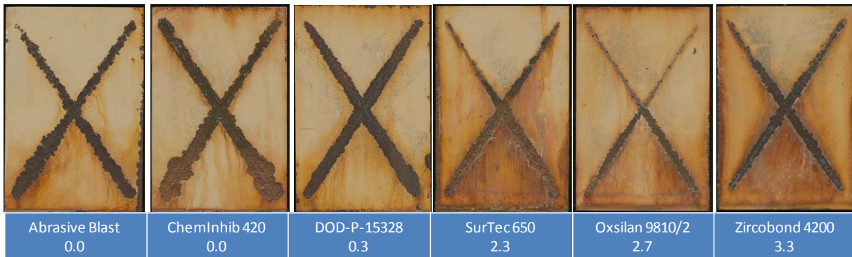
Figure 6. Average ratings of HHA test panels scraped after 80 cycles of GM 9540P with MIL-DTL-53022/MIL-DTL-53039 CARC.
