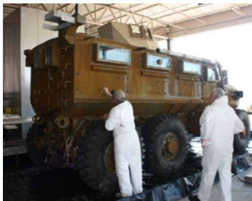
Figure 11. MRAP #1 after application of with Oxsilan 9810/2, June 20, 2011.
