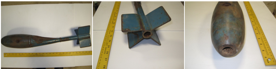
Figure 8 - Example photographs for a BDU33 25lb practice bomb showing (from left to right) a full view; a base view; and a nose view.
