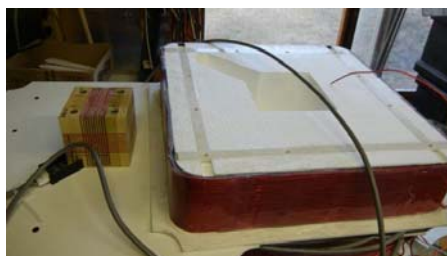
Figure 2-1 – TX/RX coil combination that forms the basis for both the MPEDEMIS and the TEMTADS 2x2
