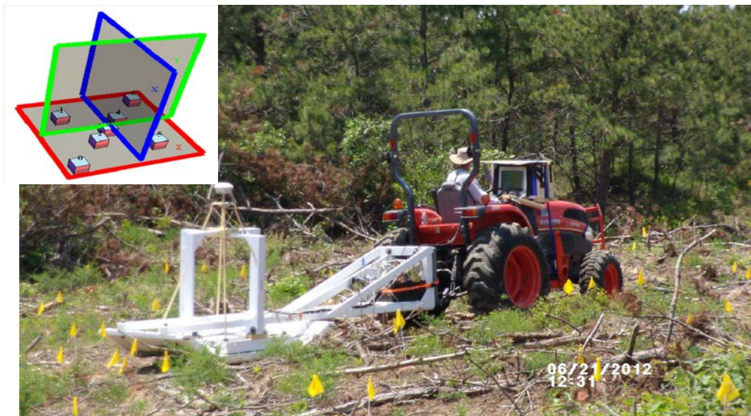
Figure 2-2: Antenna Array and Deployment of the MetalMapper at MMR
