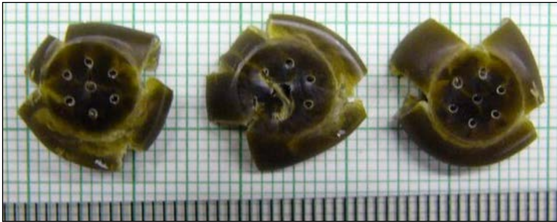
Fig. 28 Postcompression image of JA2 grain samples at a rate of \sim 100 \text{ s}^{-1} obtained at 10 \text{ }^\circ\text{C} , scale in millimeters
