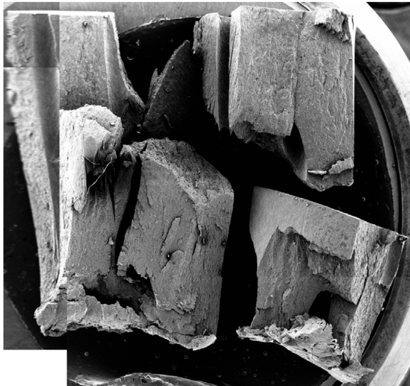
Fig. 48 SEM panorama of postcompression JA2 grain sample (uniaxially compressed at a rate of \sim 100 \text{ s}^{-1} , -50 \text{ }^\circ\text{C} , and strain greater than 40%), 10 \times magnification
