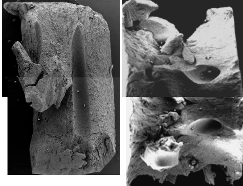
Fig. 47 SEM panorama of postcompression JA2 grain sample (uniaxially compressed at a rate of \sim 100 \text{ s}^{-1} , -40 \text{ }^\circ\text{C} , and strain greater than 40%), 50 \times magnification
