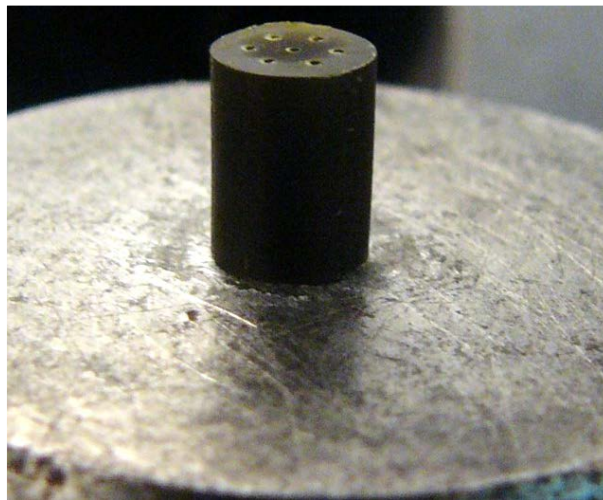
Fig. 4 Specimen loaded on stage of MTS-SHT apparatus
