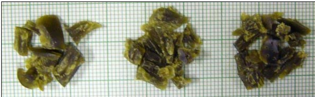
Fig. 34 Postcompression image of JA2 grain samples at a rate of \sim 100 \text{ s}^{-1} obtained at -50 \text{ }^\circ\text{C} , scale in millimeters
