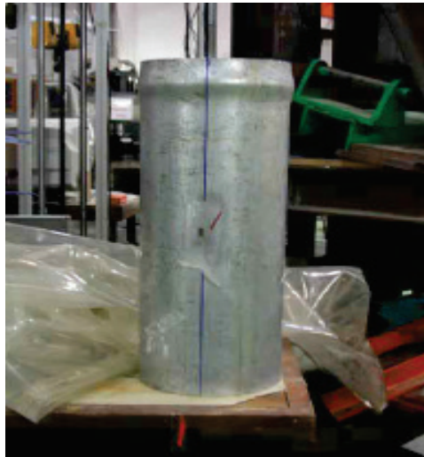
Figure 4.2. Elephant's foot buckling mode (Teng and Hu 2007).
