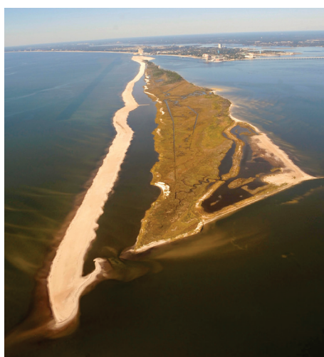
Figure 7. View of the restored shoreline and constructed lagoon with spur dike and sand weir.
