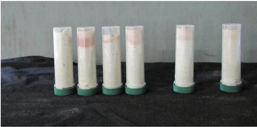
Figure 50. Photograph of Mound 3 sand samples collected after 120 min of waves at alongshore locations (from left to right): Y30, Y28, Y26, Y24, Y20, and Y18.
