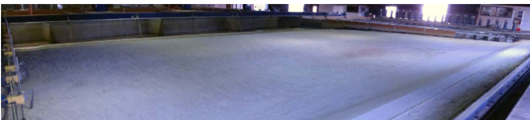
Figure 25. Panoramic view of the Mound 1 beach looking downdrift after 120 min of waves.
