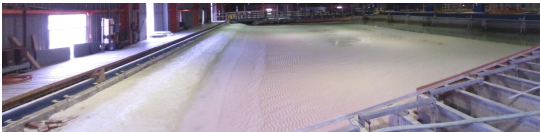
Figure 36. Panoramic view of the Mound 2 beach looking updrift after 120 min of waves.
