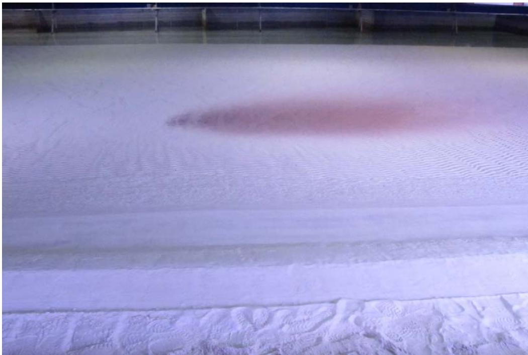
Figure 23. Mound 1 beach looking offshore after 60 min of waves.
