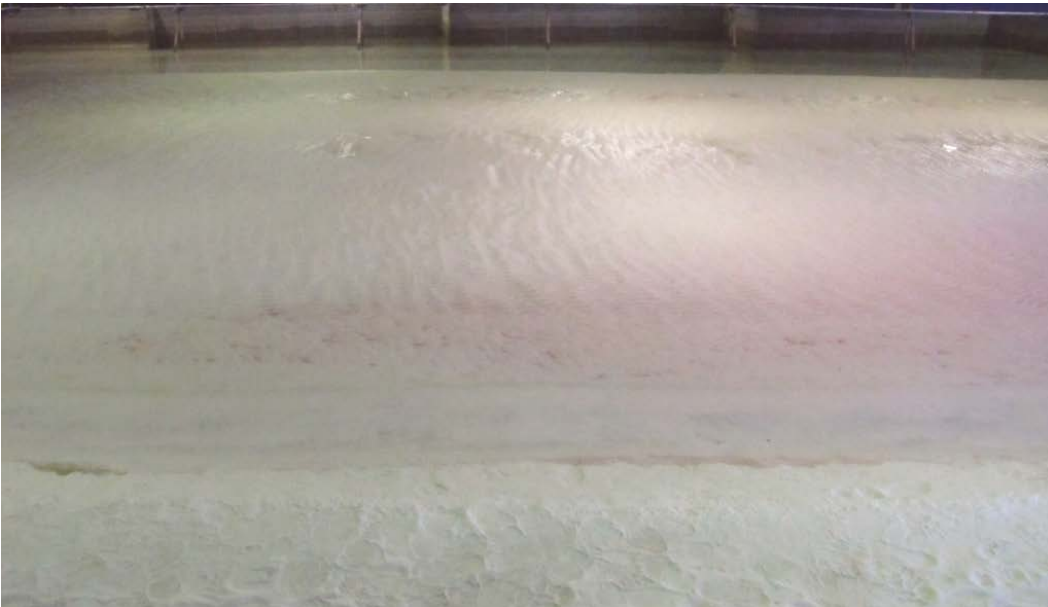
Figure 38. Mound 2 beach looking offshore after 120 min of waves.
