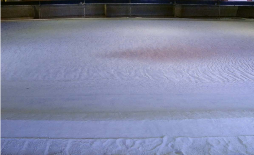
Figure 26. Mound 1 beach looking offshore after 120 min of waves.
