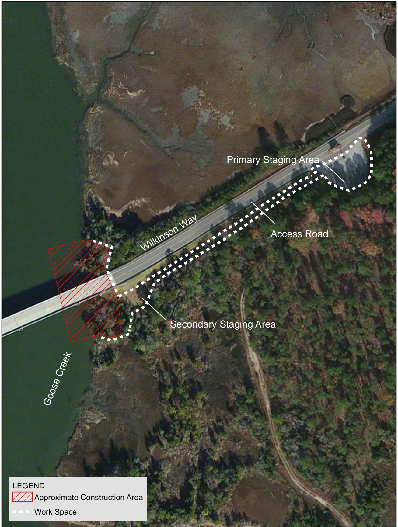
FIGURE 2-1 Work Space and Construction Area Grace Hopper Bridge Environmental Assessment Joint Base Charleston - Weapons Station
