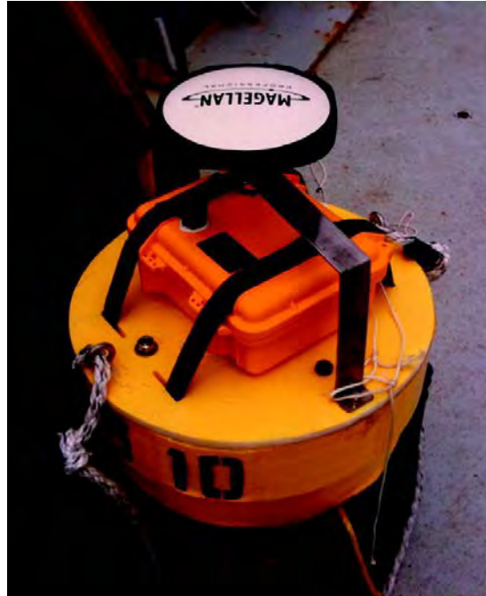
Figure 3. Prototype wave resolving drifter (WRD) (from Herbers et al. 2012).
