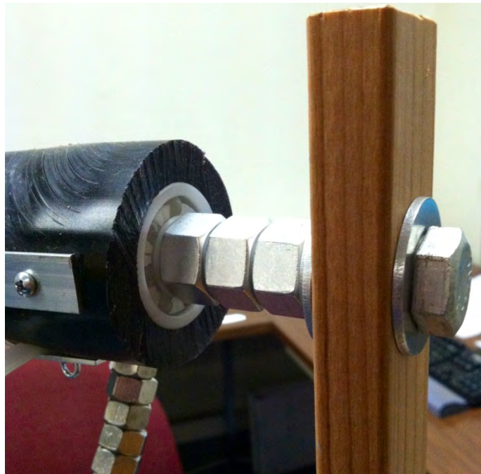
Figure 19. SWOMS cradle arm, hardware, bearing, and tubing.
