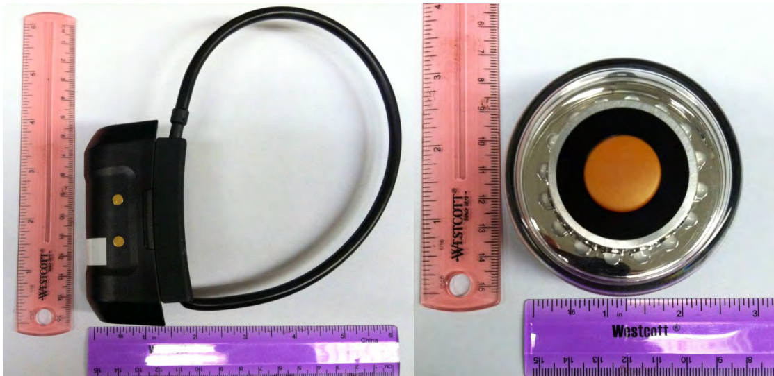
Figure 7. (left) Garmin DC 40 GPS-enabled transmitter. (right) NaviSafe marine light.
