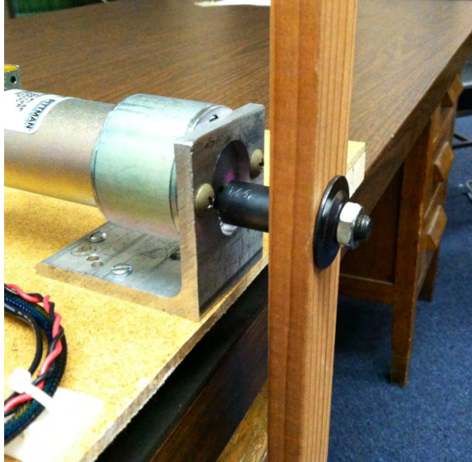
Figure 15. SWOMS rotational arm secured to motor shaft.
